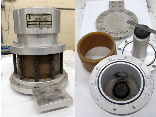
Fig. 5 L3 Communications ST-300 spark gap switch
