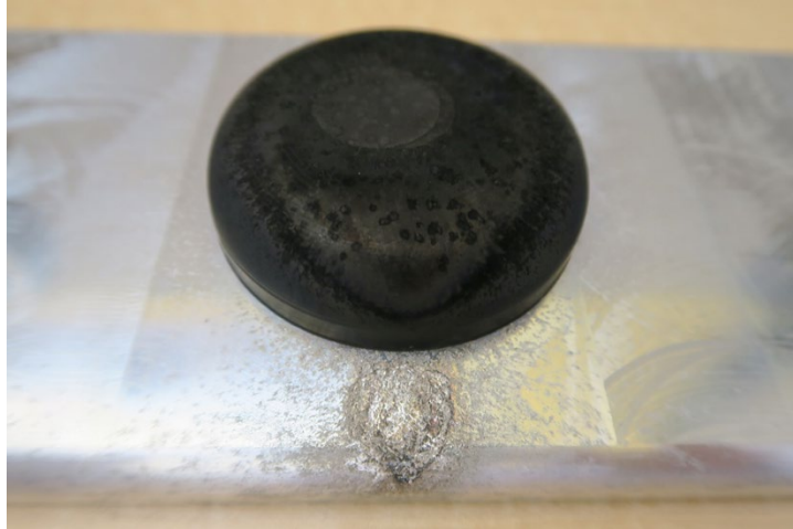
Fig. 21 Evidence of J \times B forces acting on the arc in the spark gap switch
