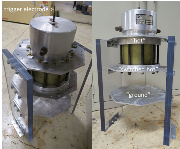
Fig. 6 Modified L3 Communications Model ST300 spark gap switch
