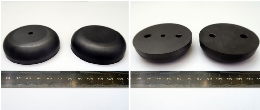
Fig. 8 Graphite electrodes used in the ARL spark gap switch (scale in millimeters)
