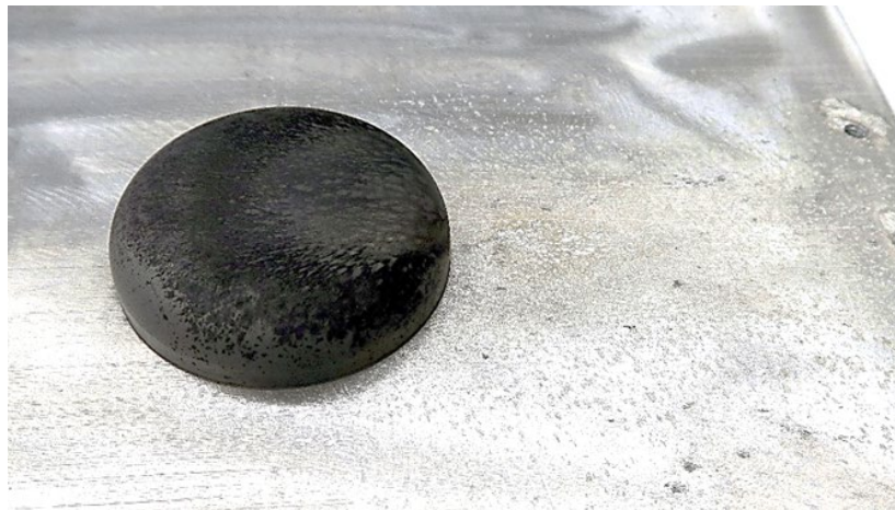
Fig. 12 Negative graphite electrode after initial testing
