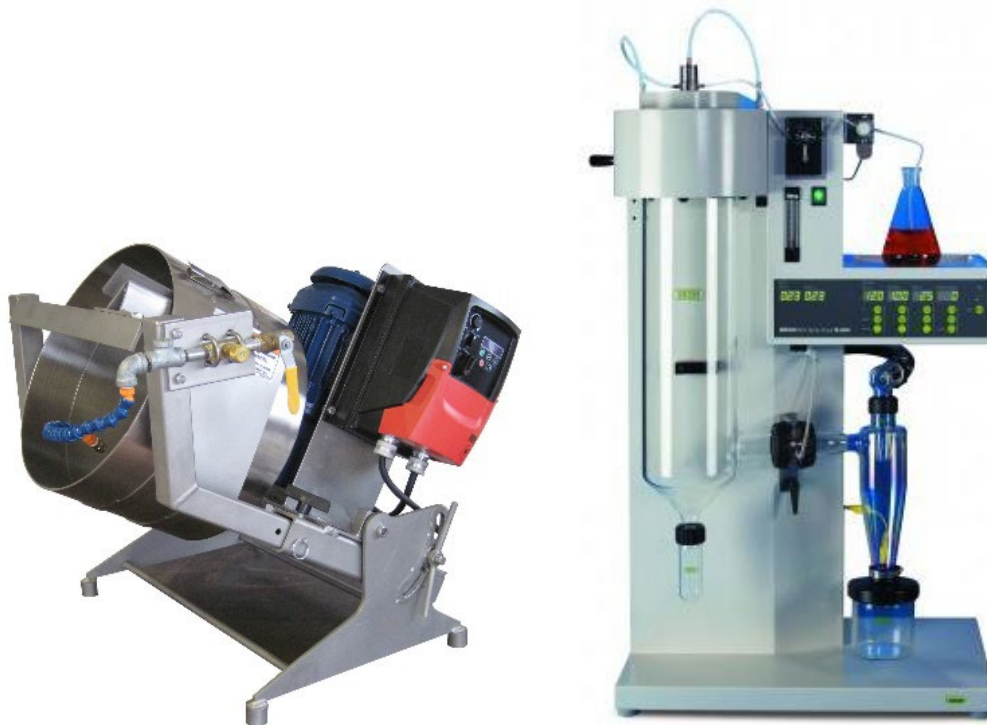
Fig. 1 Mars Mineral DP-14 pan granulator and the Buchi B-290 spray drier used in the SiC granulation experiments
