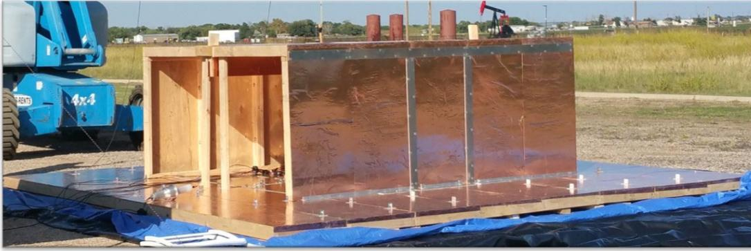
Figure 31. Full-scale prototype ESA used to test gain, pattern, and direct drive feasibility.
