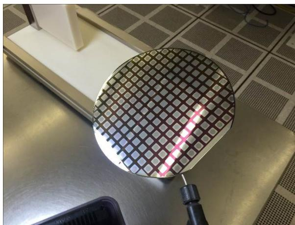
Figure 18. Picture of the entire SiC wafer while being processed to produce the PIN PCSSs. The wafer diameter is 150 mm.
