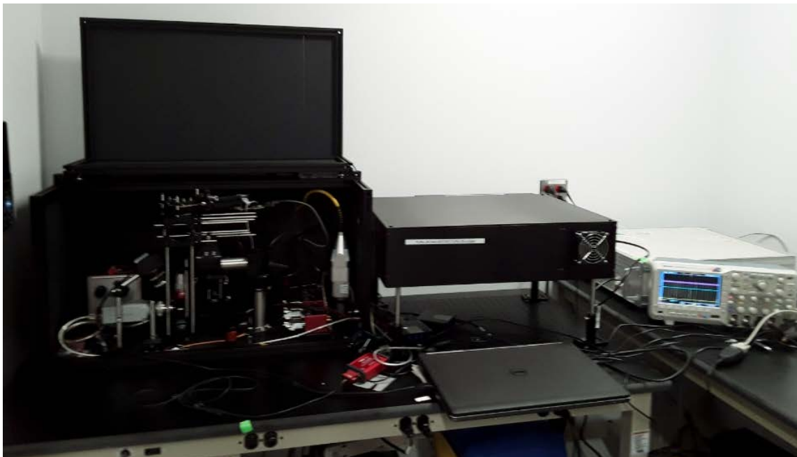
Figure 5. Image of the on-site BioLP. We have assembled a prototype biolaser printer at our facility. We used the printer to deposit cells into the gel constructs printed with our extrusion (Cellink ) bioprinter.
