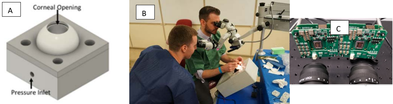
Figure 10. The tissue holder with the tracking system electronics integrated as a “patient head”. The surgeon (B) sutures the corneal construct placed within the tissue holder (A). The tissue holder is placed into the gray box (arrow) which represents the patient head. The gray box houses the electronics shown in C.
