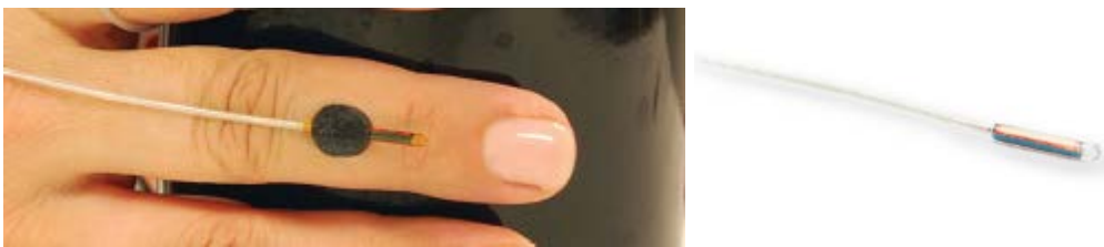
Figure 9b. The micro sensor is a 1.8 mm outer diameter magnetic sensor which is on a flexible cable. The device can be easily mounted to forceps with an adhesive or fixing pad.
