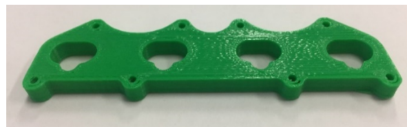
(b) Engine intake flange printed by FDM
