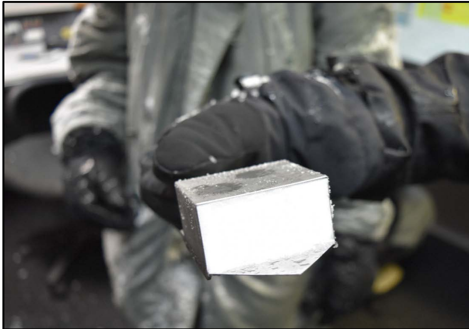
Figure 4. Snow density measurement sample. Sampling tool of known volume and weight.
