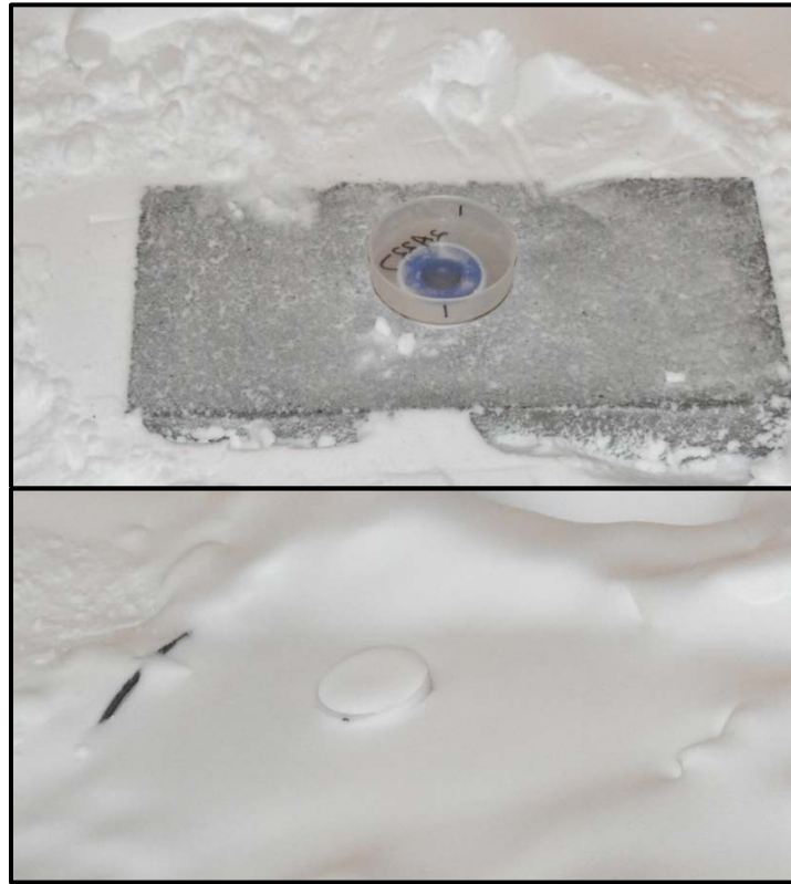
Figure 5. Snow density sampling technique, dish of known volume and weight.
