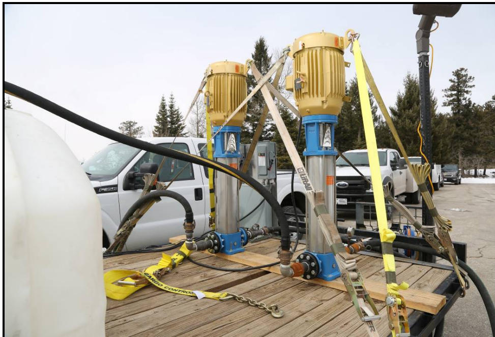
Figure B-4. Booster pump (53 gallons per minute, operational) - Goulds Model 10SV19GK4C60. One pump per snow machine.
