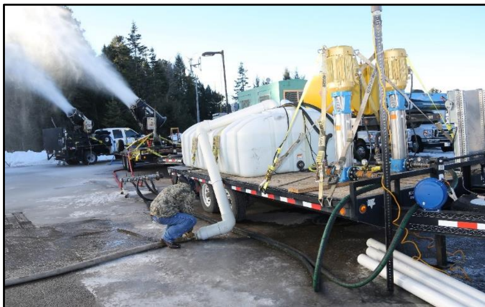
Figure 2. Water reservoir tank and trailer mounted booster pumps. Snow making machines operating in the background.
