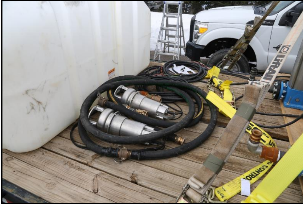
Figure B-3. Sump pump - Ebara Model 50DWXU61.54. Sump pumps feed standing reservoir water to booster pumps. One pump per booster pump.
