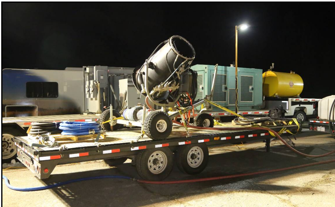
Figure 3. Example of integrating mobility to the snow machine for easy movement.
