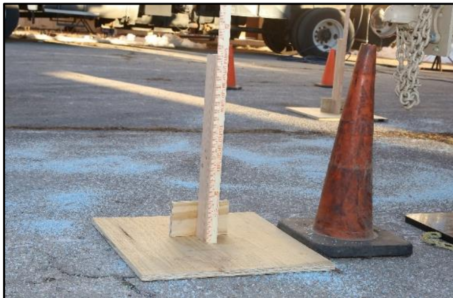
Figure 8. 16 x 16 inch wood base with yard stick mounted for snow measurement.
