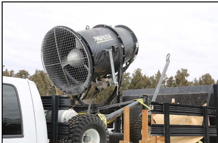
Figure B-1. Snow Machine SMI Standard PoleCat***, 18 nozzles and 15 horsepower fan.
