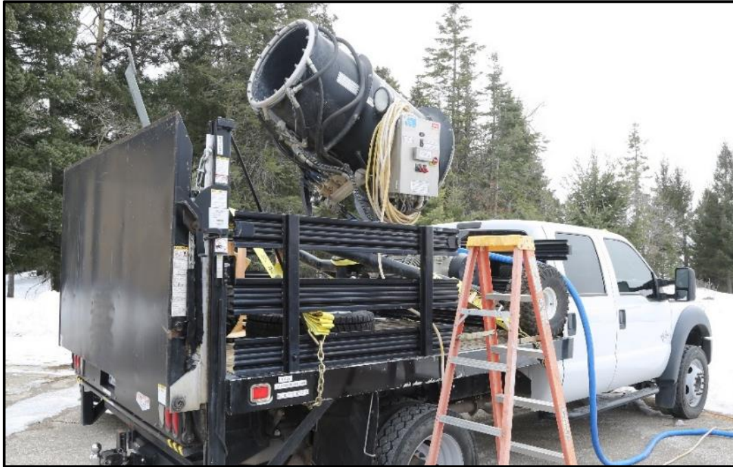
Figure 4. Example of integrating mobility into the snow machine for easy movement.
