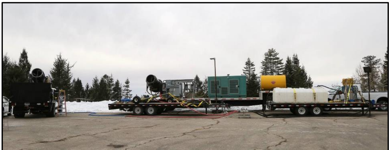
Figure 6. Snow test setup showing two snow making machines, generator, and trailer with water reservoir tank with mounted booster pumps.
