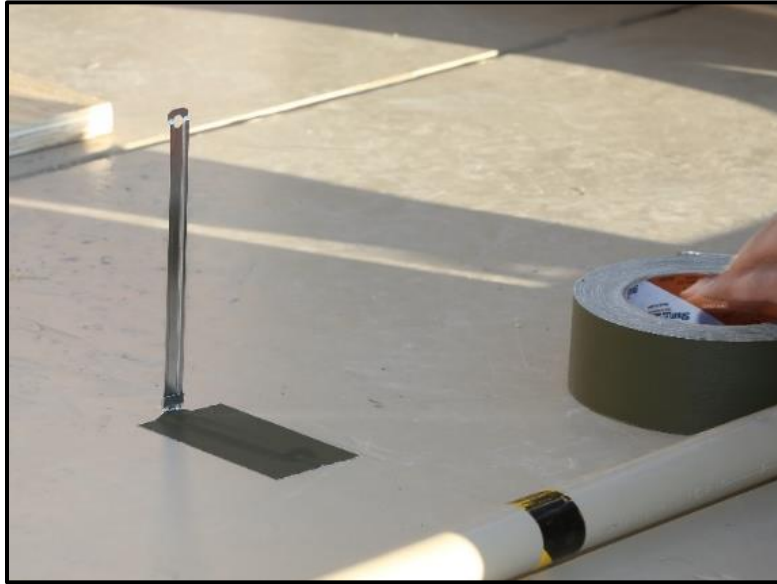
Figure 7. Snow depth gauge mounted on test item surface.
