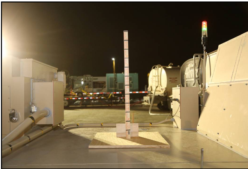
Figure B-12. Snow depth gauge (large), 16 x16 inch wood base with yard stick mounted for snow measurement.
