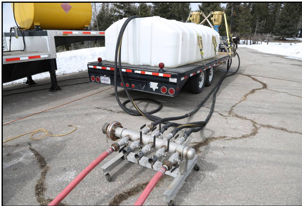
Figure B-8. Water hose connections from booster pump to manifold with emergency return to reservoir tank.
