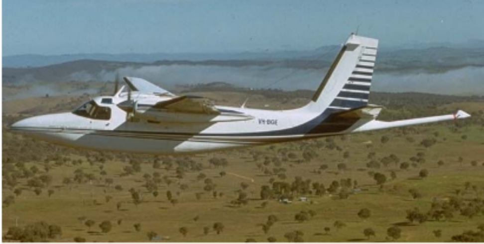
Figure 6: Fixed wing aircraft with stinger seen extending beyond the rudder. [4]
