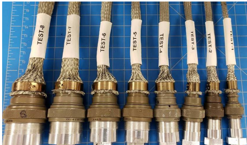
Figure 2. Test Article Before Tensile Testing (e.g. Test articles 1-8)
