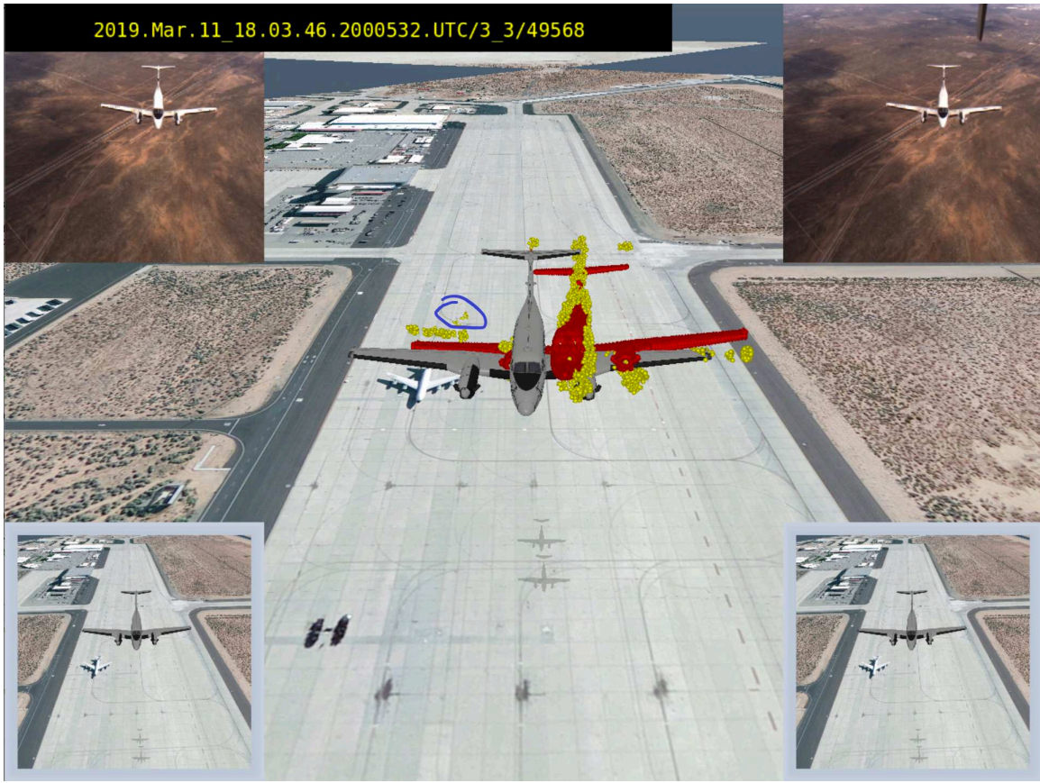
Figure 28: Relative Pose Estimation With Indicated Outliers
