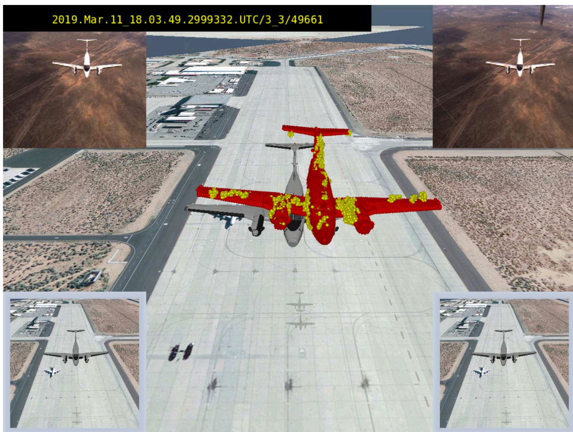
Figure 17: Sample Relative Pose Estimation Result from Calibrations in Figure 16
