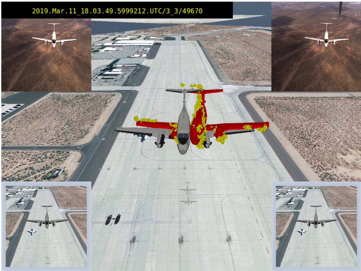
Figure 23: Relative Pose Estimation for Flight 3.3 After Camera Calibration Adjustment
