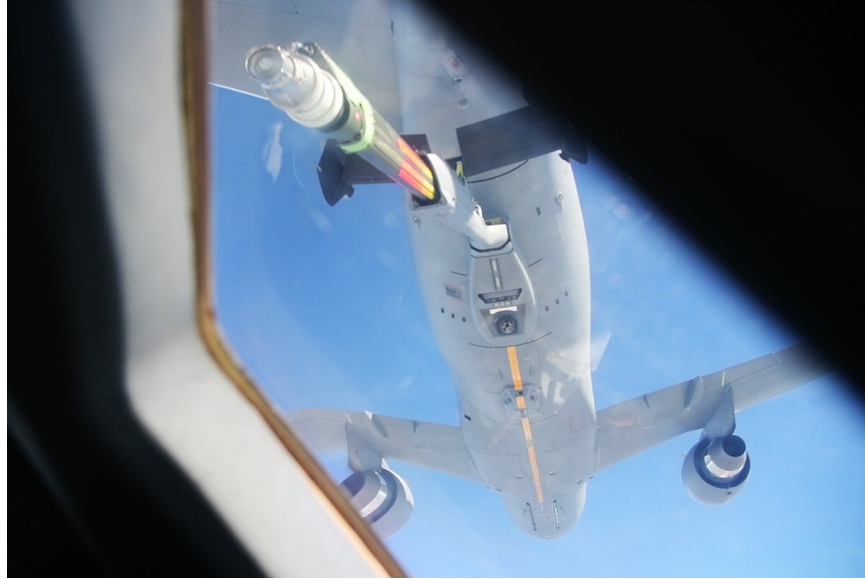
Figure 4: KC46 Camera and Boom Placement [29]
