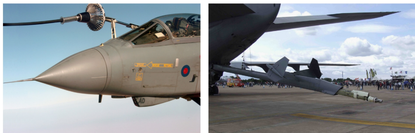
Figure 1: Refuelling methods: (Left) probe-and-drogue and (Right) boom [1]
