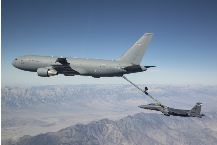
Figure 3: Aerial refueling connection: KC-46 boom to fighter receptacle [23]
