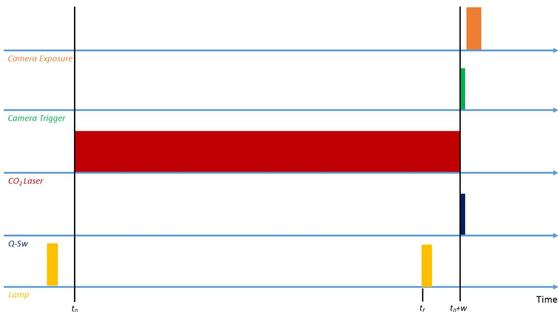
**Figure 69.** TCTI pulsed laser heating time scheme.
