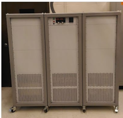
Figure 5. (a) Magna Power M series 250 kW DC power supply; (b) a schematic of the power feeding circuit of ACT-II.
