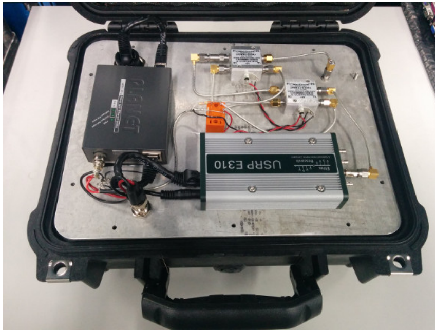
Fig. 22 Ruggedized field TM receiver internal component layout
