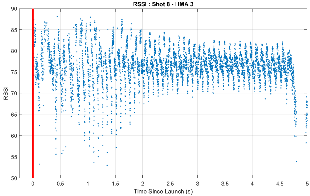
Fig. 25 Graph of RSSI vs. time for HMA 3 mid-range TM receiver
