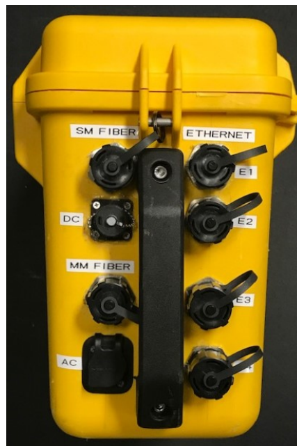
Fig. 18 Picture of the exterior connectivity of the assembled field network switch
