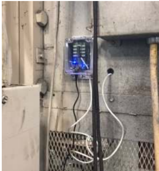
Figure 6. Retrofit kit attached to 400 ton press at Steelcase.
