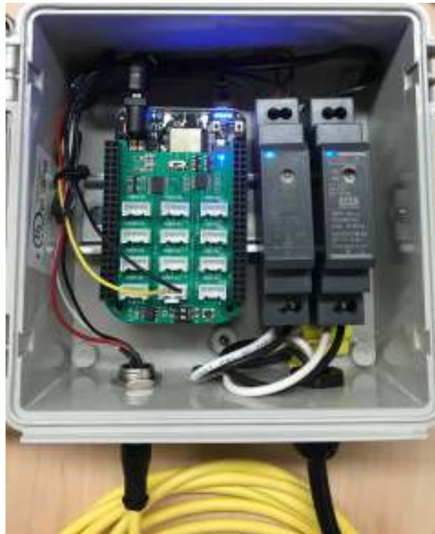
Figure 7. The second generation of the retrofit kit with DIN rail mounted devices and standardized connectors.
