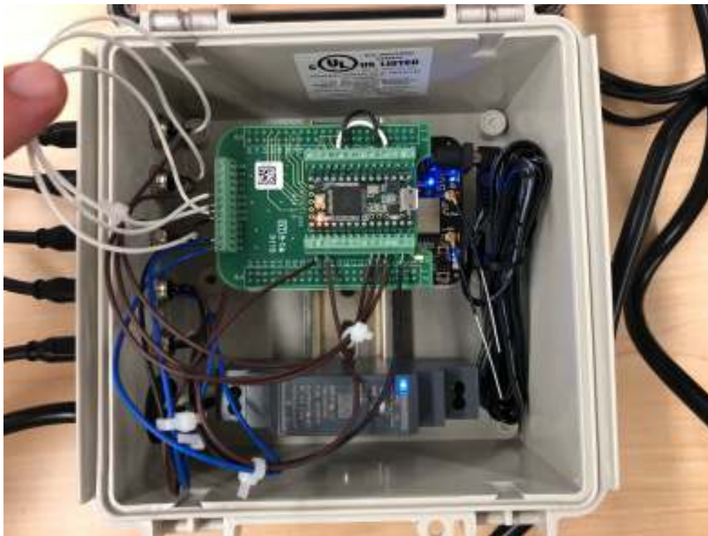
Figure 9. The third generation retrofit kit with custom BBBW cape (green board).
