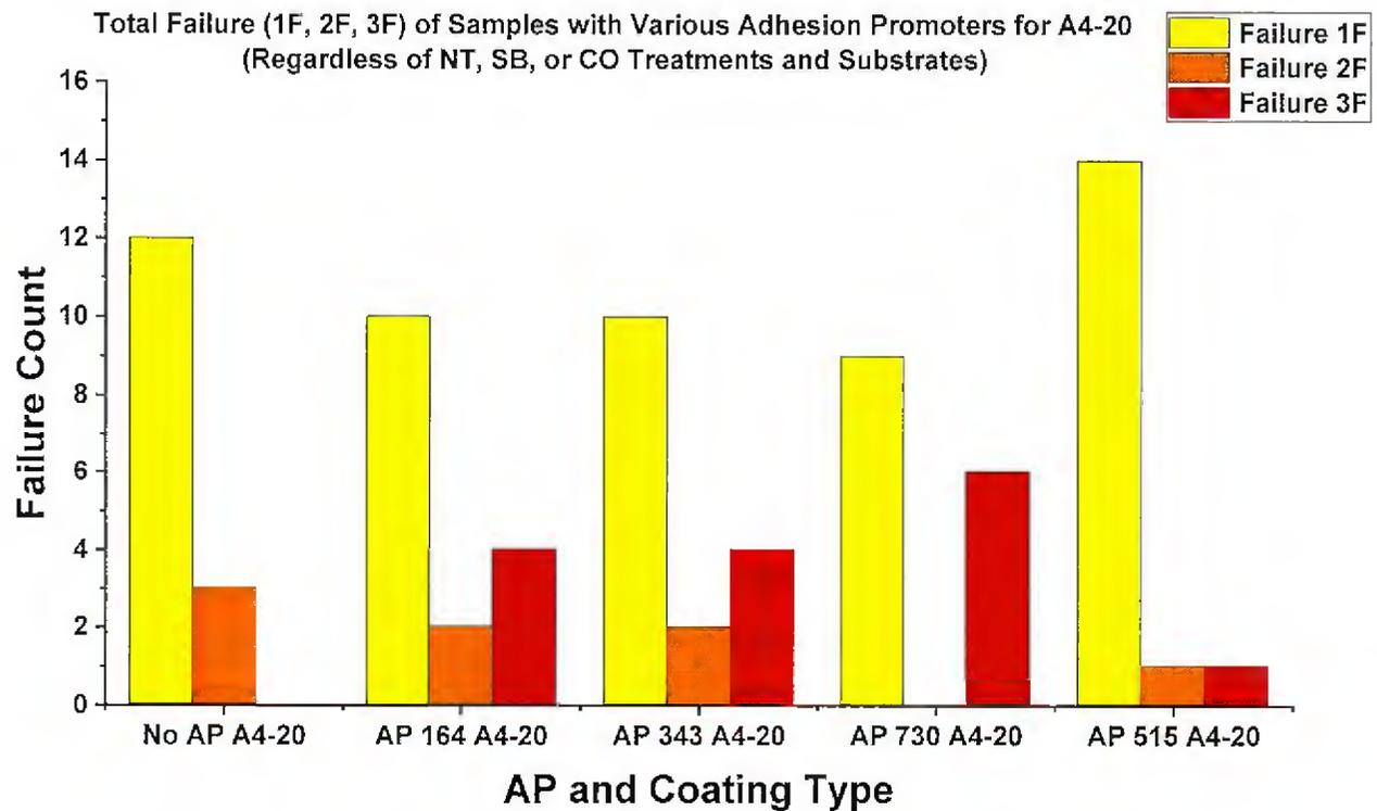
**Figure II.17:** Total failure count of A4-20 coatings between different adhesion promoters.
