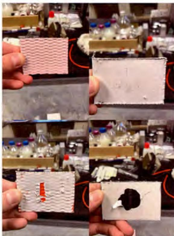
**Figure II.10:** Top left to right: 0F, 1F failure classification. Bottom left to right: 2F, 3F failure classification
