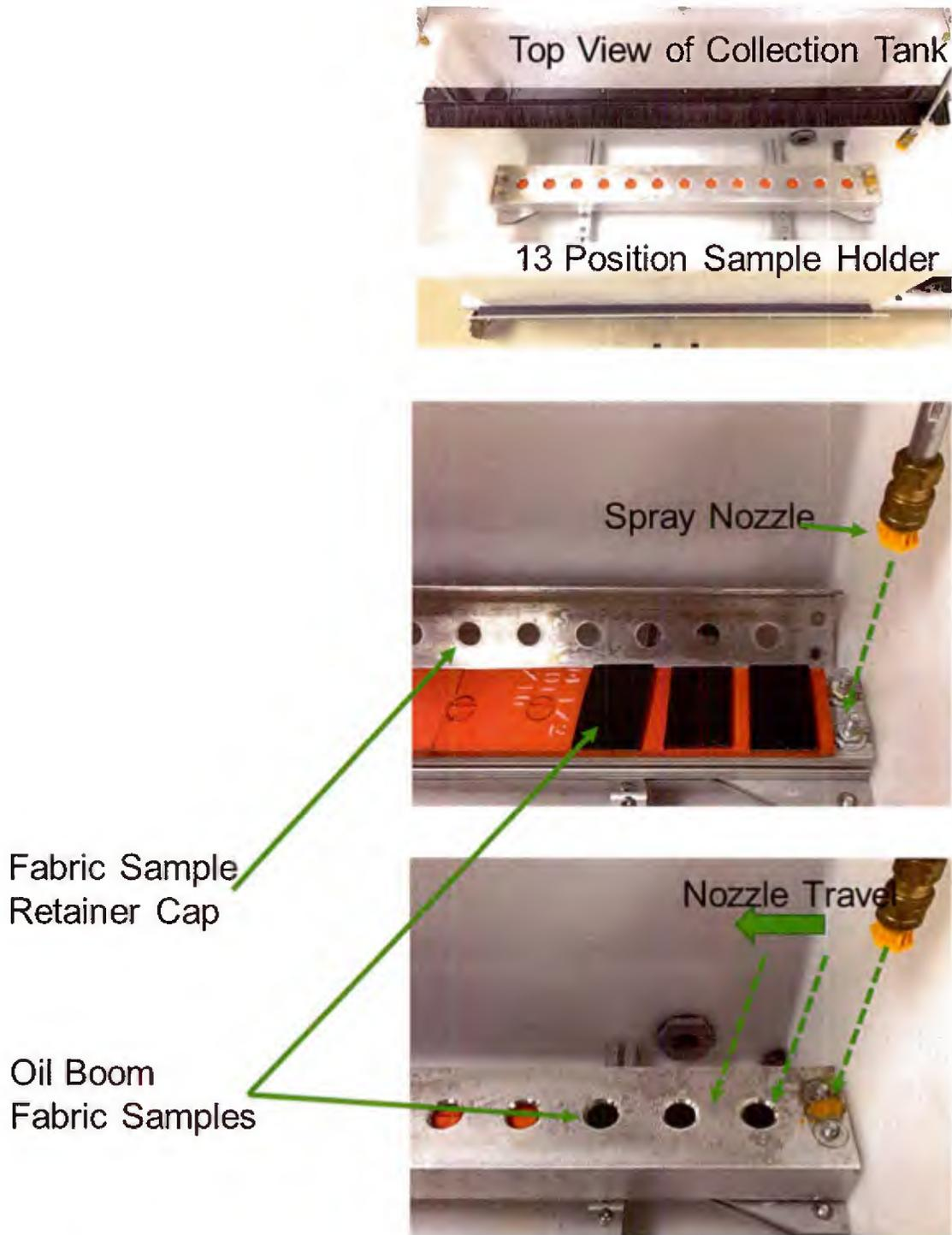
**Figure II.9:** Pictures showing the distance of nozzle from the substrates, 13-sample holder itself, and direction of nozzle travel (photo credits – James Bahr)
