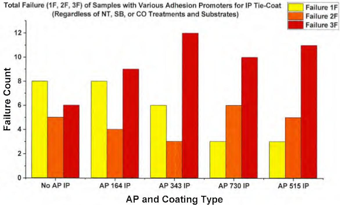
Figure II.18: Total failure count of IP tie-coat coatings between different adhesion promoters.
