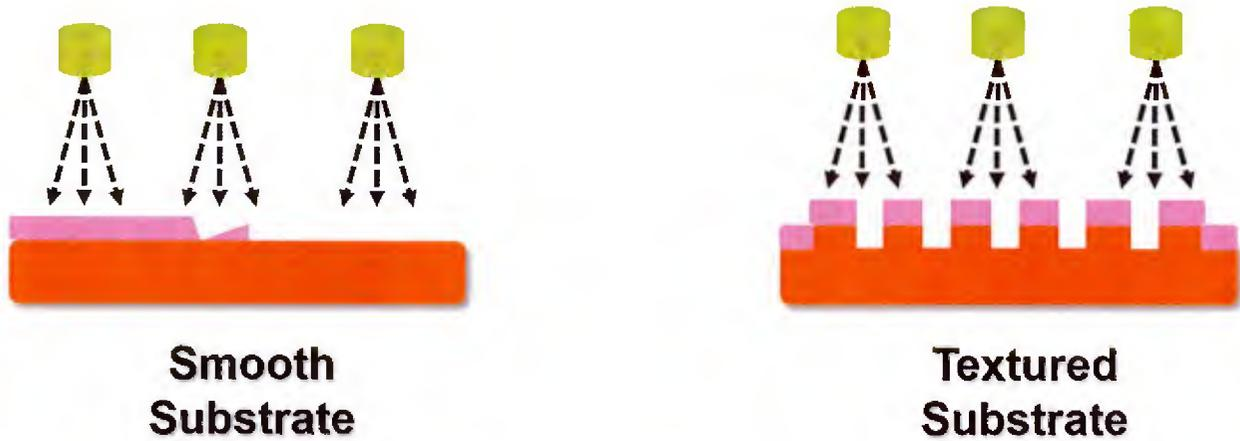
**Figure II.25:** On smooth substrates, once coating damage occurs the forces of water penetrate under the film more readily, leading to quicker complete delamination. On textured substrates more force is directed into pockets of the substrate and coating on the ridges is less susceptible to adhesion loss and damage.
