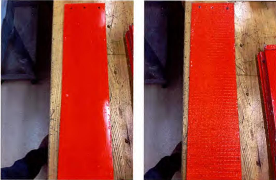
**Figure II.27:** Left; Smooth substrate #1 coated with transparent A4-20. Right; Textured substrate #2 coated with A4-20
