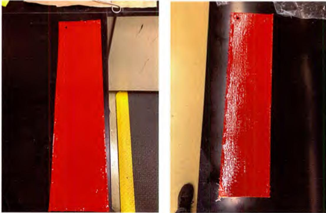
**Figure II.29:** Left; Smooth substrate #1 coated with topcoat Hempasil X3+. Right; Textured substrate #2 coated with topcoat Hempasil X3+
