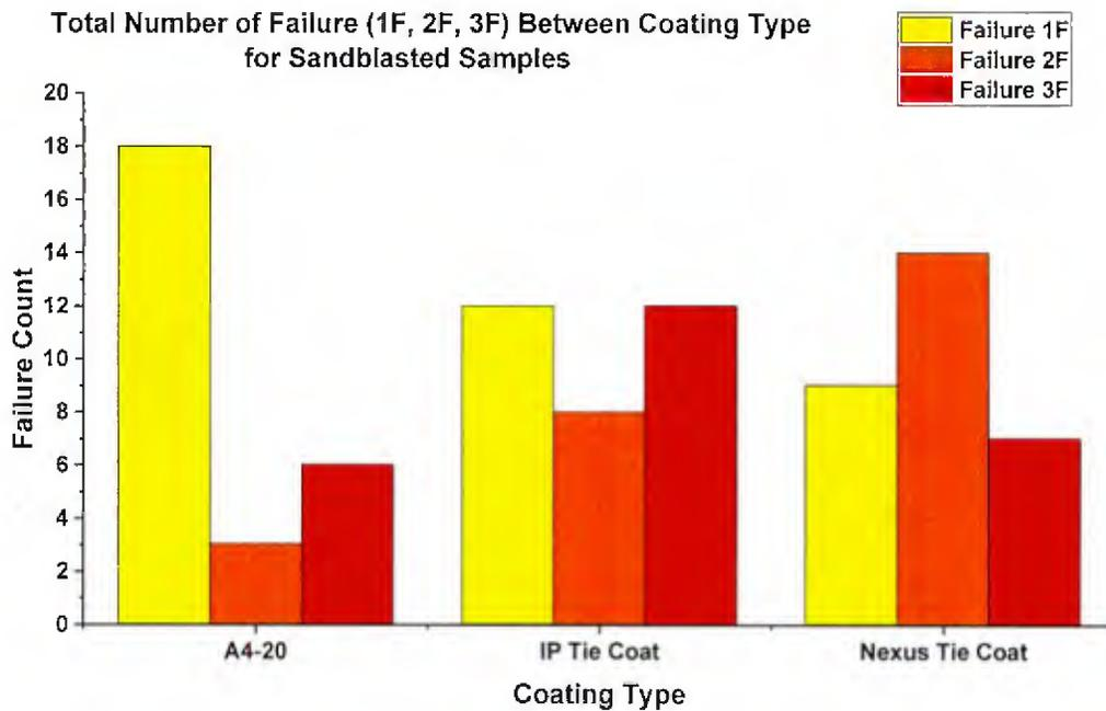
**Figure II.21:** Total number of failures between different coating types for sandblast treated samples.
