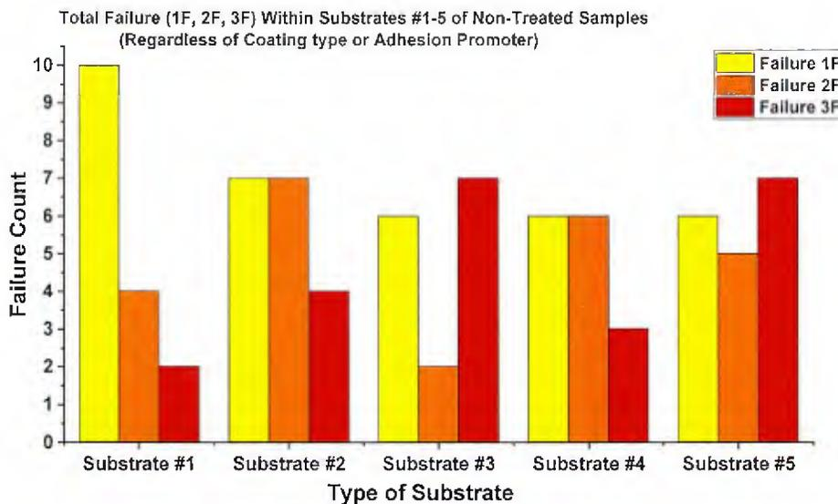
**Figure II.14:** Total number of failures of non-surface treated samples regardless of coating type or adhesion promoter
