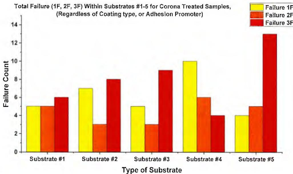
Figure II.16: Total number of failures of corona treated samples regardless of coating type or adhesion promoter.
