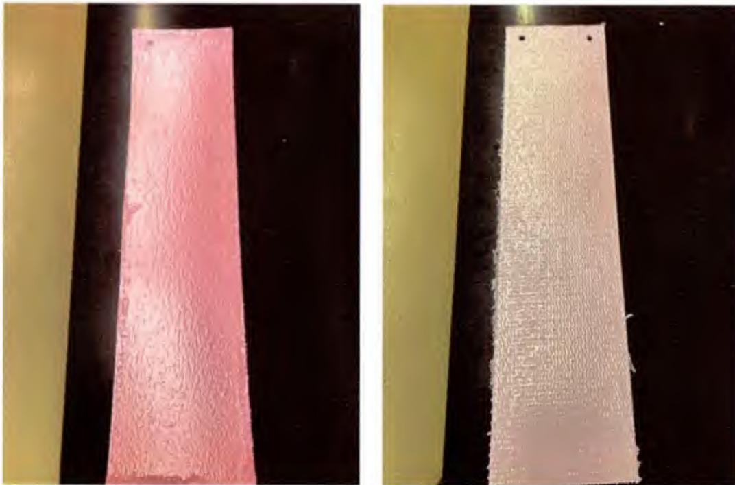
**Figure II.28:** Left; Smooth substrate #1 coated with Nexus tie-coat. Right; Textured substrate #2 coated with Nexus tie-coat
