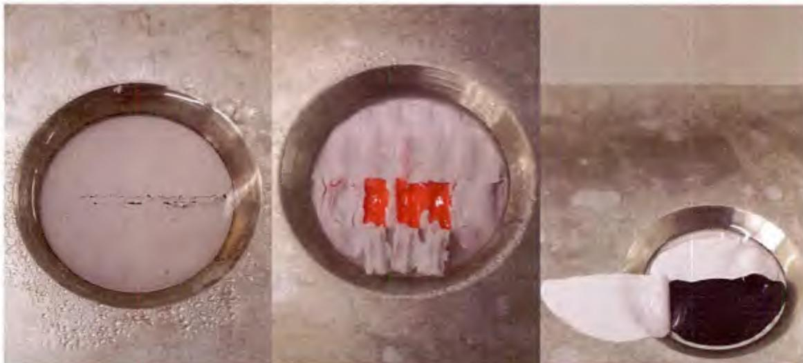
**Figure II.12:** From left to right: IP 1F, IP 2F, IP 3F failure classifications
