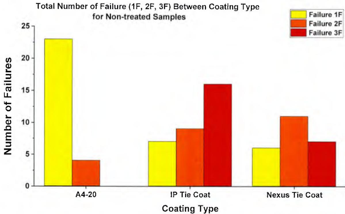
Figure II.20: Total number of failures between different coating types for non-surface treated samples.
