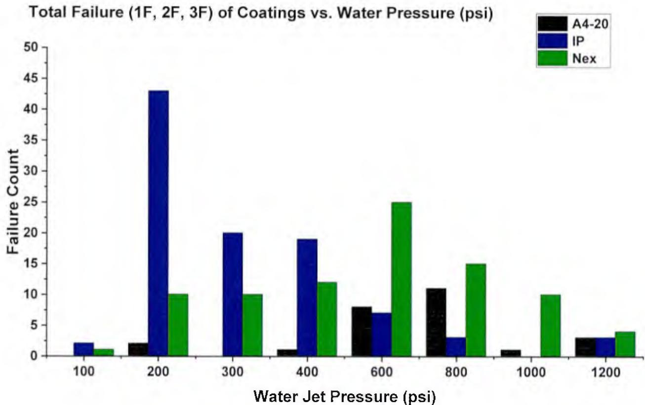
**Figure II.23:** Total failure counts (1F, 2F, 3F) for the different coating types at increasing pressures regardless of substrate, surface treatment, or adhesion promoter.
