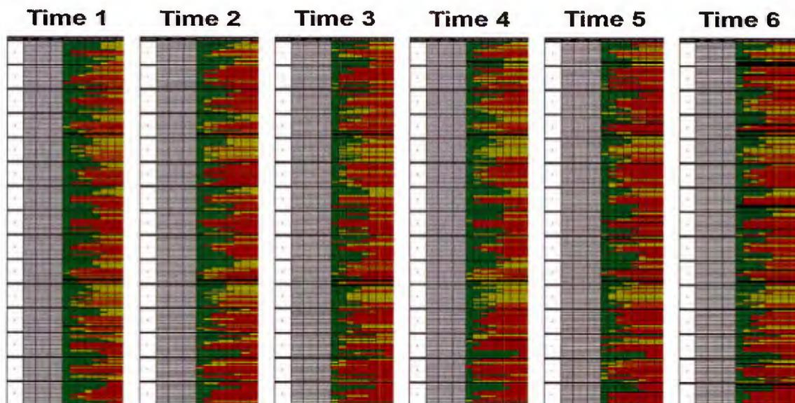
**Figure II.24:** Data from all independent variables are entered against water pressure. Color-coding of failure categories 0F, 1F, 2F, and 3F are green, yellow, orange, and red. Time periods 1-6 were all entered this way and offer a quicker method for picking out trends in increased adhesion performance
