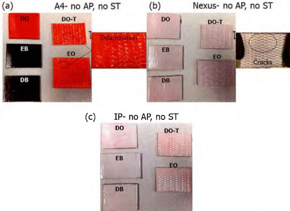
**Figure II.5.** Images of fabric samples with no surface treatments and no APs, coated with (a) A4-20, (b) Nexus, and (c) IP. Abbreviation ST indicates surface treatment.
