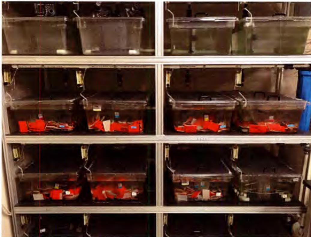
**Figure II.7:** All 1350 samples placed in circulating water tanks
