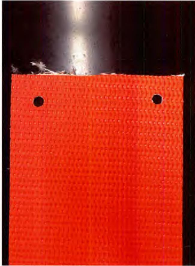
**Figure II.26:** A cut sample with holes punched out for mounting
