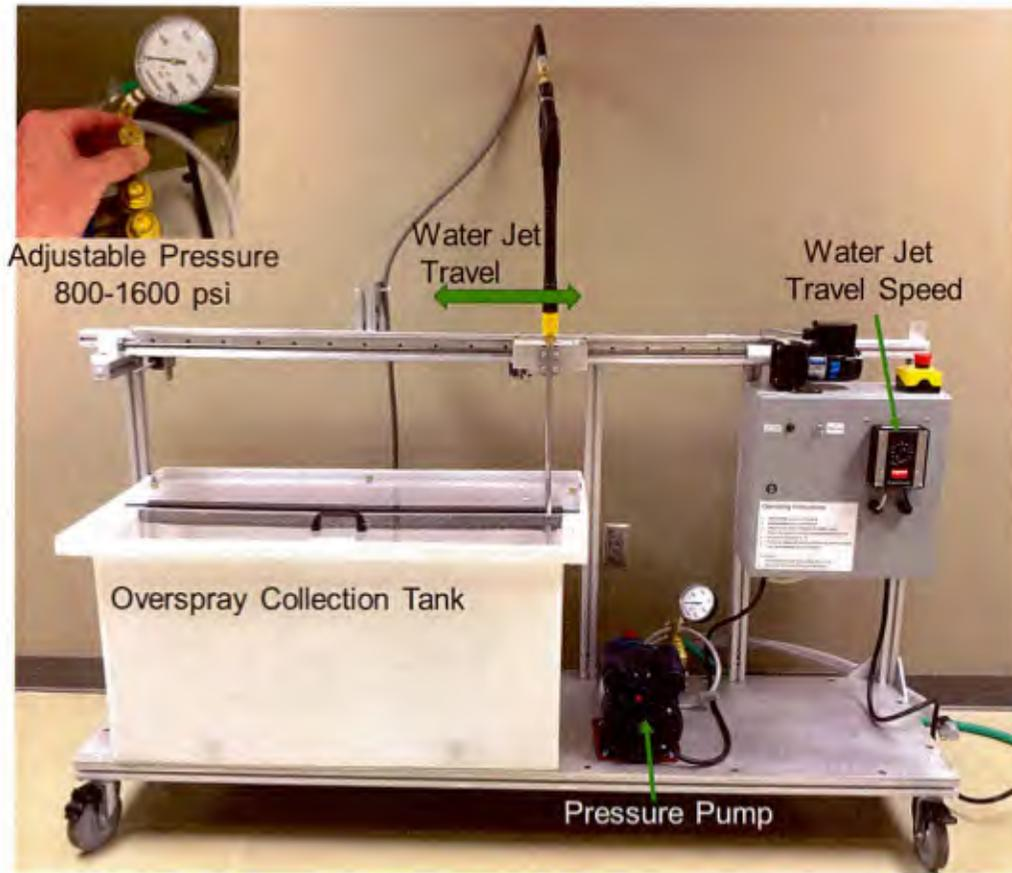
Figure II.8: Custom adhesion testing apparatus showing max pressure, direction of travel and variable speed control (photo credits – James Bahr)
