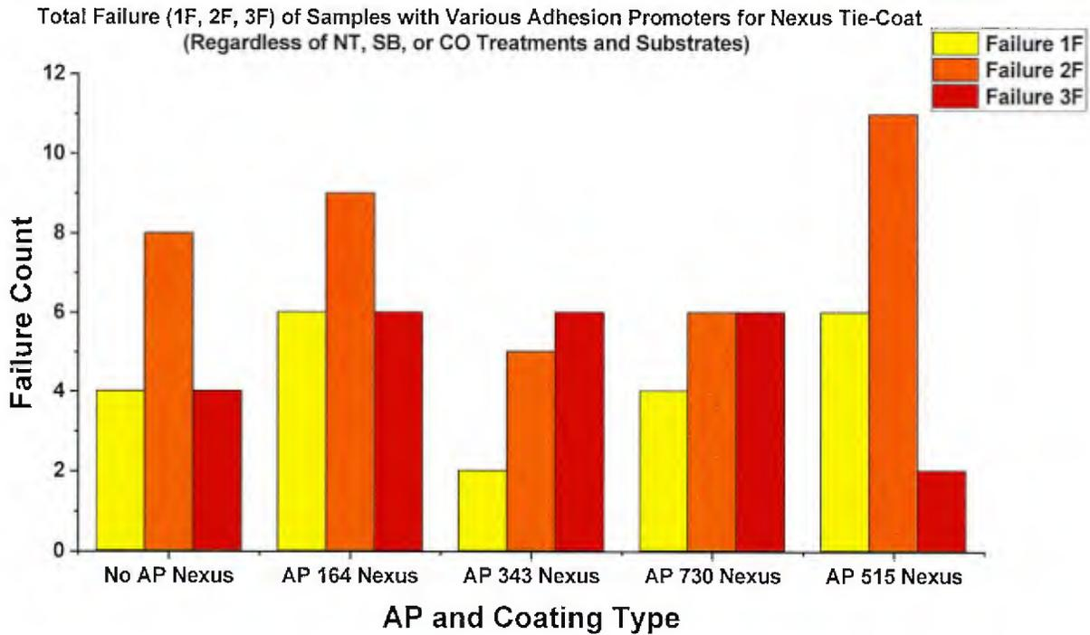
Figure II.19: Total failure count of Nexus tie-coat coatings between different adhesion promoters.
