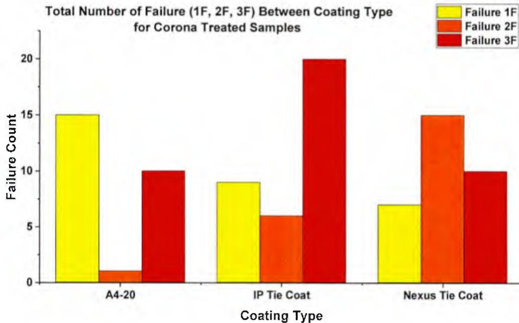
**Figure II.22:** Total number of failures between different coating types for corona treated samples.
