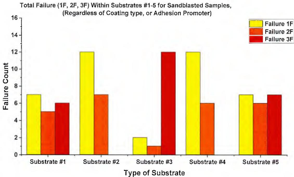
Figure II.15: Total number of failures of sandblast treated samples regardless of coating type or adhesion promoter
