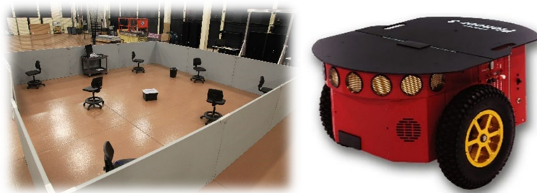
Figure 1: Pioneer robot and playpen test area for the neuromorphic reactive controller, ControlNet.
