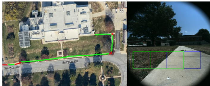
Figure 2: The path followed by the Pioneer robot using OluNet running on the IBM TrueNorth neuromorphic processor (left). An image showing the sub-patches passed to the TrueNorth for classification. The green patches are identified as grass, while the blue patch is classified as concrete.
