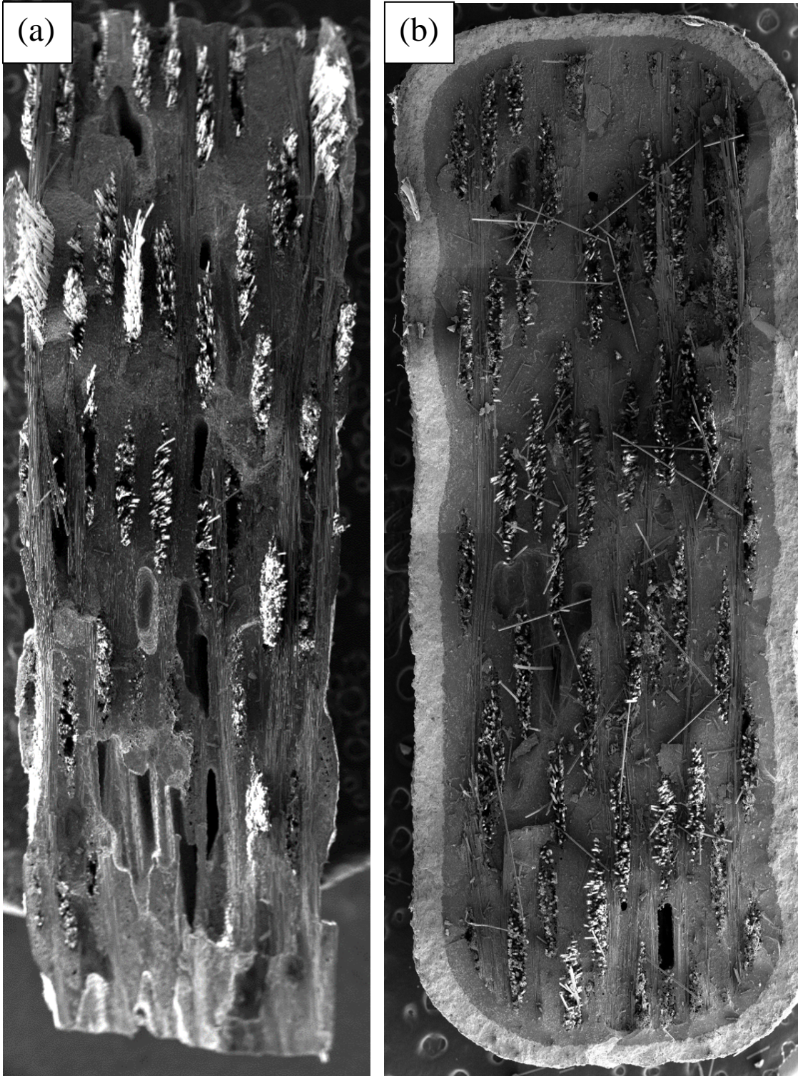
Figure 4.28: Micrographs of uncoated Hi-N/MI-SiC (a) compared to EBC/Hi-N/MI-SiC (b). Both specimens were subjected to fatigue testing at 1200°C and reached run-out ( N_f > 200,000 cycles) in steam
