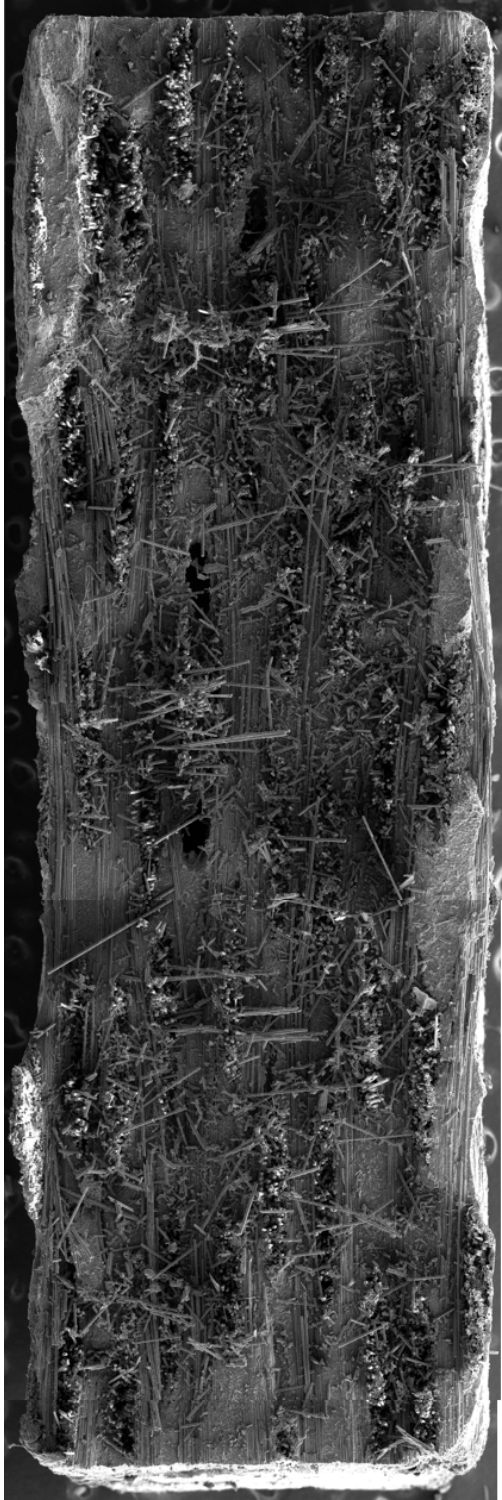
Figure 4.16: Hi-N/MI-SiC/Grit-Blasted specimen P15006-4, Tensile Test. Micrographs show significant fiber pullout with little oxidation.
