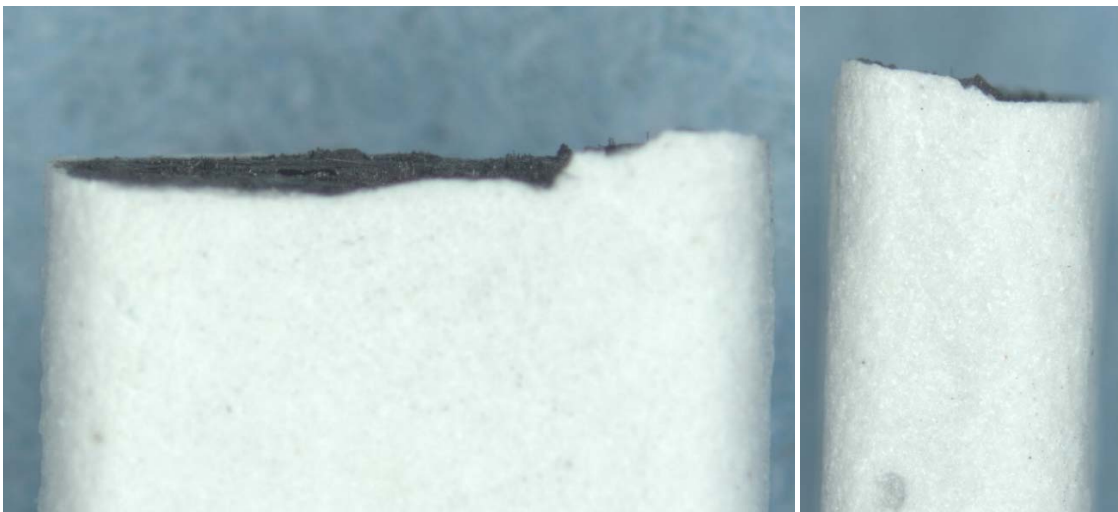
Figure 4.18: Optical micrograph of specimen P15002-7 subjected to tension-tension fatigue testing to failure at 1200°C in air. \sigma_{\max} = 130 MPa, N_f = 8,869 cycles
