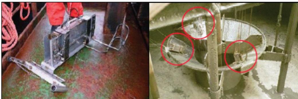
There was a concern that turbulence generated around the sampler's opening meant that the flow into the sampler was not likely isokinetic, which may bias the sample. Additionally, this method appeared to be
