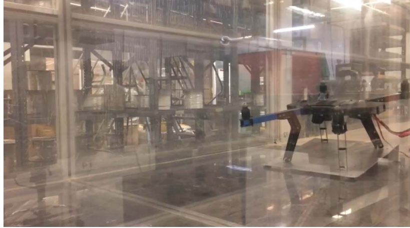
Figure 14. MURPHEE Flow Visualization with Rotors On
