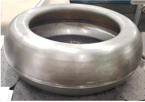
(a) Liner prior to hole machining
