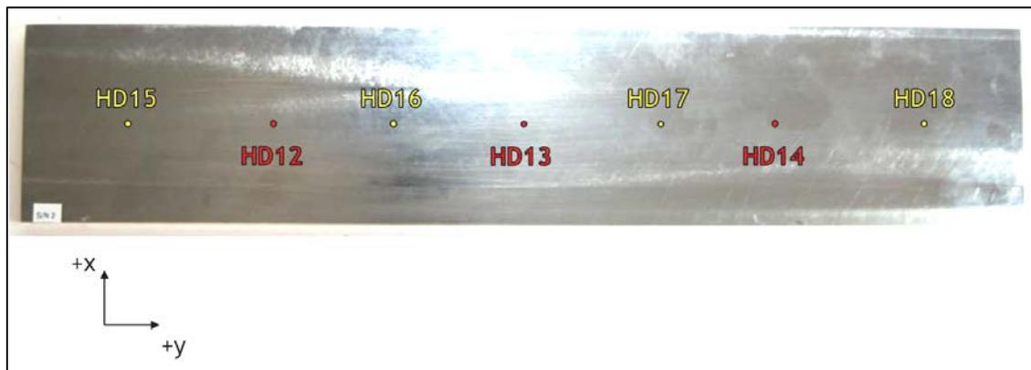
**Figure 26: Representative titanium plate and hole-drilling locations (LSP treated spots in yellow and far field baseline locations in red) [105]**
