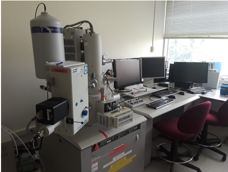
Figure 10. The SEM, EDS and accompanying computers used for the experiment.
