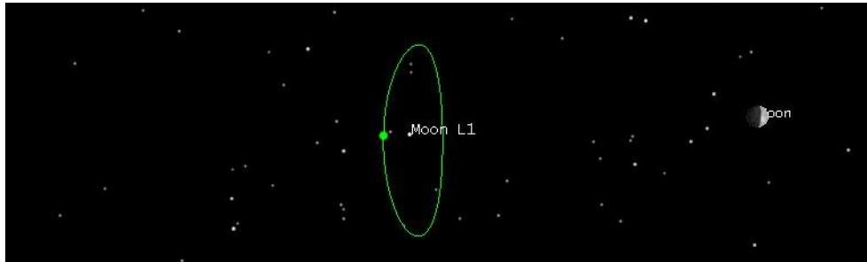
Figure 4: Lyapunov orbit in STK for A_{y'} = 15,000 km and A_{z'} = \mathbf{0} km with \phi = \mathbf{180^\circ}, \psi = \mathbf{0^\circ}
