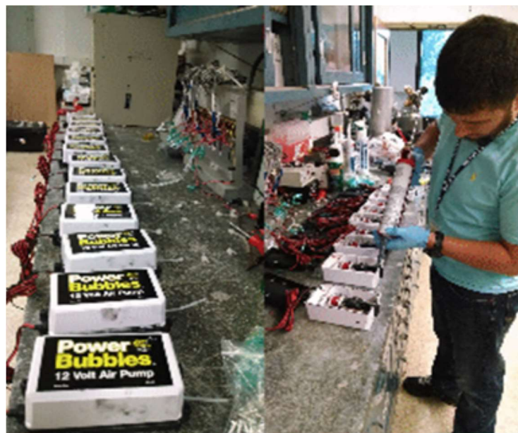
Figure 8. Well headspace gas recirculating pumps, sealed
