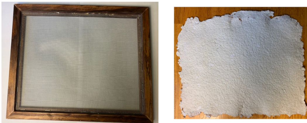
Fig. 27 Photos of homemade papermaking deckle and the sample of paper produced
