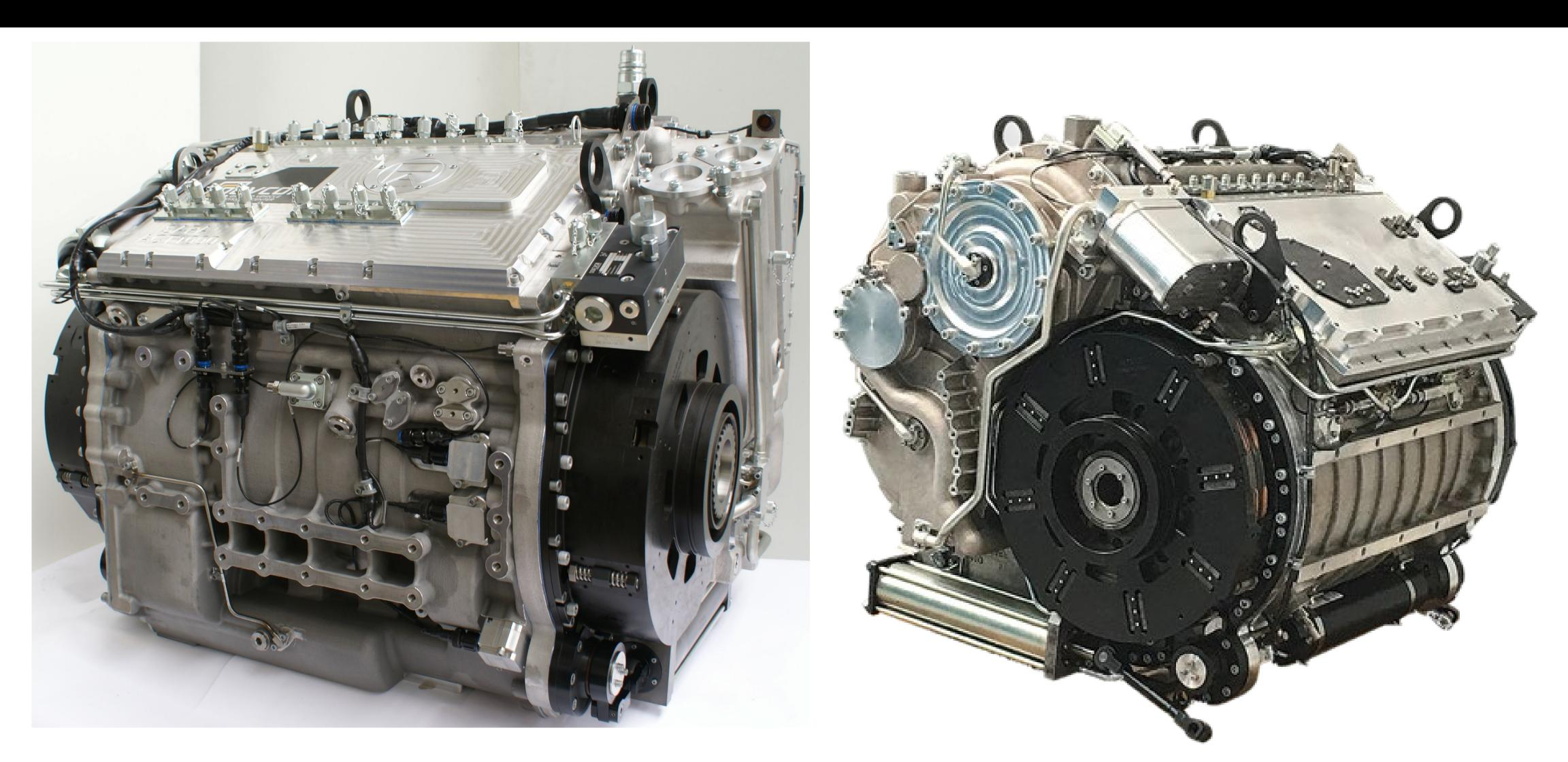
The Advanced Combat Transmission is a family of high power density transmissions that employ a new 32-speed cross-drive design. This new transmission design removes or replaces the most inefficient elements of a conventional cross-drive transmission with highly efficient gears, improving transmission efficiency in even the worst situations to over 90%.
