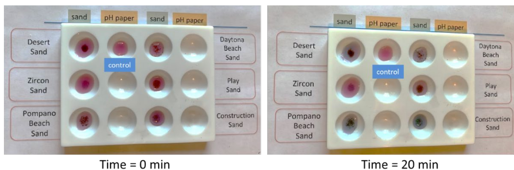
Fig. 24 Testing the pH of sand specimens with the cabbage juice indicator. At time = 0 min, the indicator for all samples and the control solution is pink. At time = 20 min, the indicator color for several specimens turned blue, indicating that they are alkaline.
