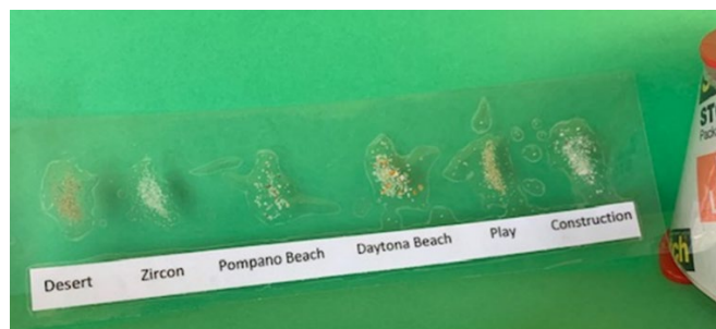
Fig. 9 Sand specimens for microscopic analysis prepared by encasing in transparent, heavy-duty packing tape
