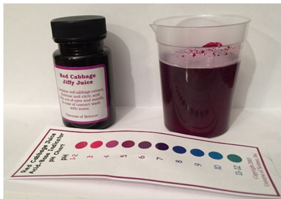
Fig. 22 Commercially available dried cabbage juice extract, reconstituted with water (right). Color/pH chart shown at bottom.
