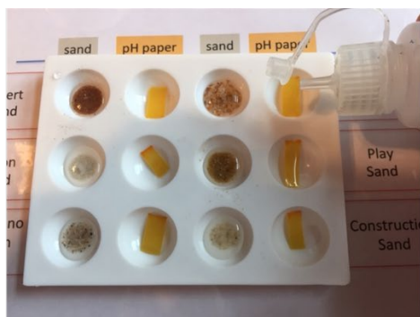
Fig. 19 Preparation of samples for pH testing
