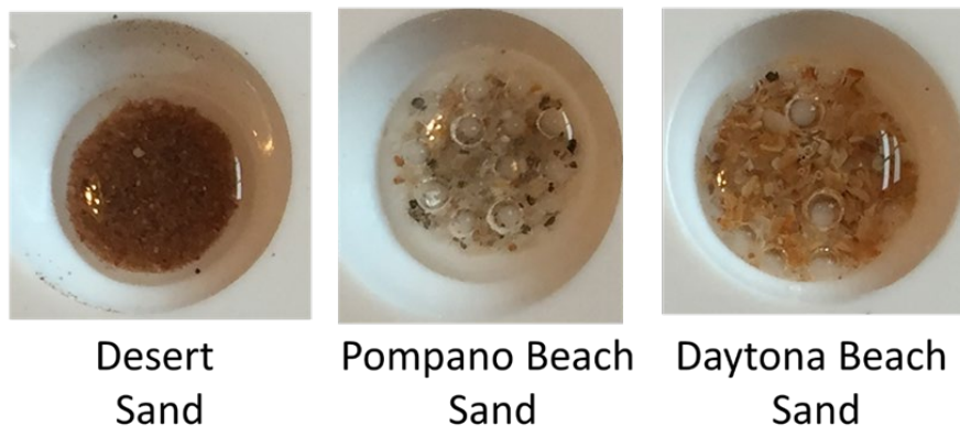
Fig. 16 Evidence of bubbling from CO 2 generation observed for the desert and beach samples
