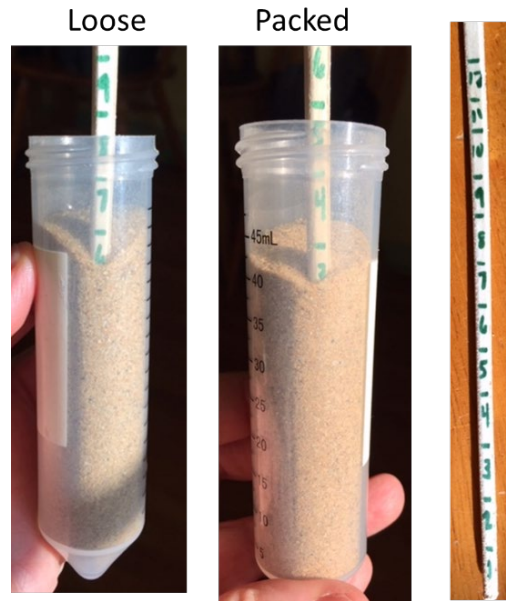
Fig. 11 Play sand (assumed to be river sand) loosely packed (left) and compacted (right). Distance into the sand to which a stick may be inserted is limited by inter-particle interactions.
