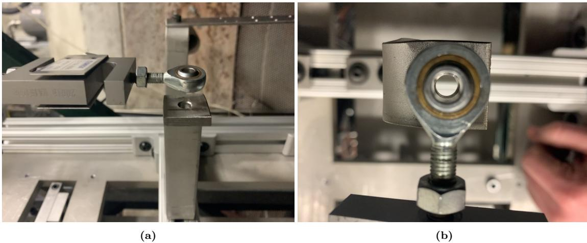
Figure 60. Flexure-based thrust stand calibration load cell connection alignment: (a) side-view of attachment, (b) vertical alignment of load cell connection with engine mount.
