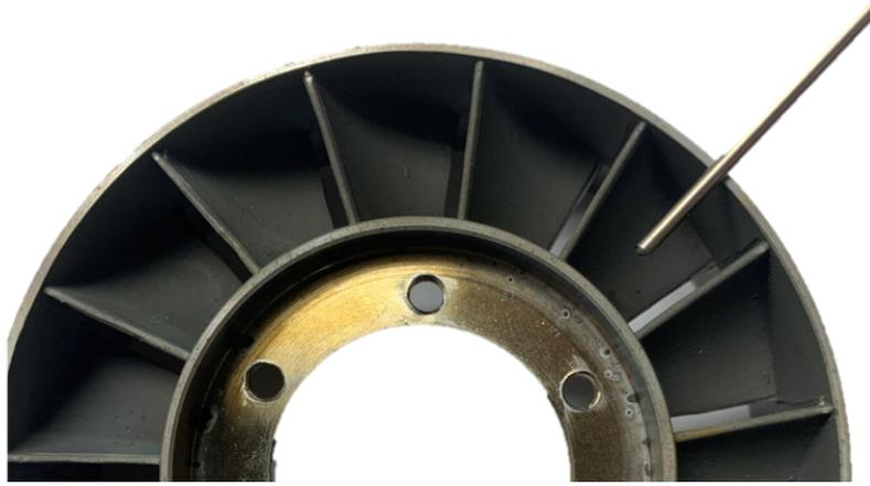
**Figure 71. Thermocouple positioned in front of NGV, illustrating relatively large size of the thermocouple to the passage size.**
