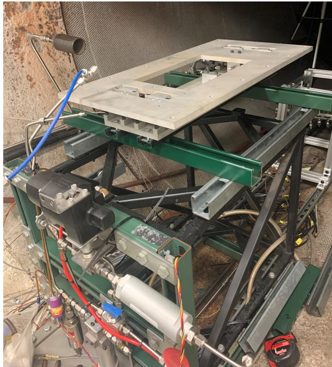
**Figure 51. Installation of new, flexure-based thrust stand.**
