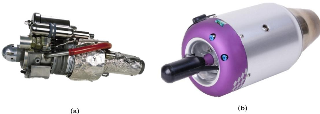
**Figure 1. Microturbine turbojet engines: (a) Hamilton Sundstrand TJ-50 used on the ADM-160 MALD, (b) commercially available, civilian engine.**
