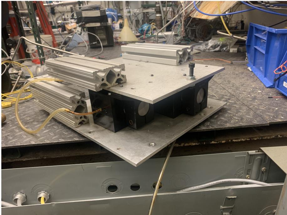
Figure 50. Air-bearings used to support pre-existing thrust stand.
