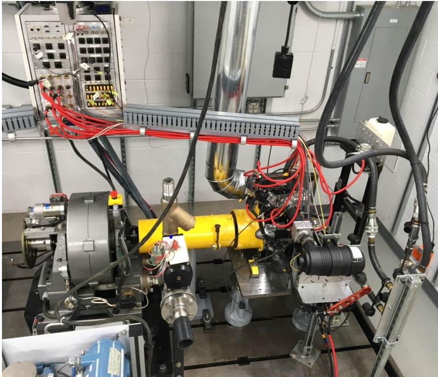
Figure 1: Test cell showing dynamometer, driveline, engine, and data acquisition system
