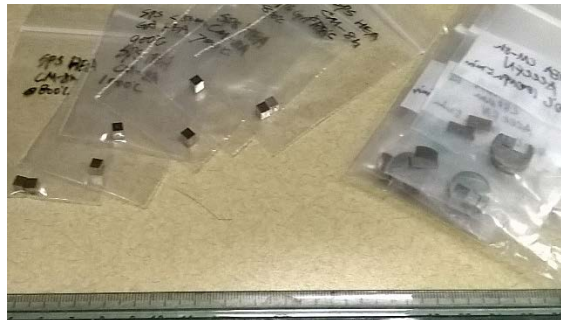
Fig. 3.4.5: SPS-processed AlCoCrCuFeNi HEA disks and the cubic samples by EDM.
