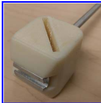
Fig. 4 Link block fitted with slider and link rod. The diagonal slot fits onto the drone frame.
