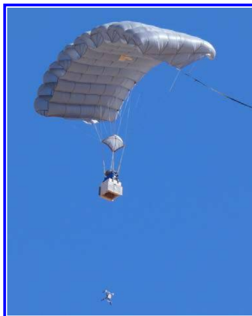
Fig. 2 Automated Drone Delivery from Airdrop Systems (ADDAS) prototype during flight test.
