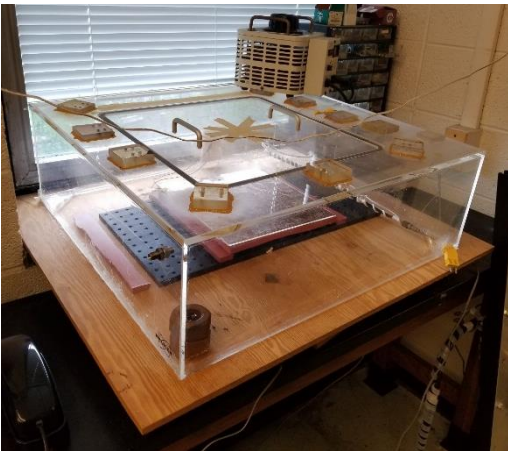
Fig. 5. The casting table has a heated casting surface for evaporation of solvent. The enclosure T is also controlled. The slurries are cast using the doctor blade (right side).
