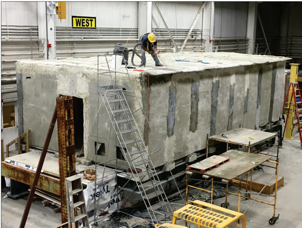
Figure 1. Overall view of constructed indigenous material TCB shortly before testing.
