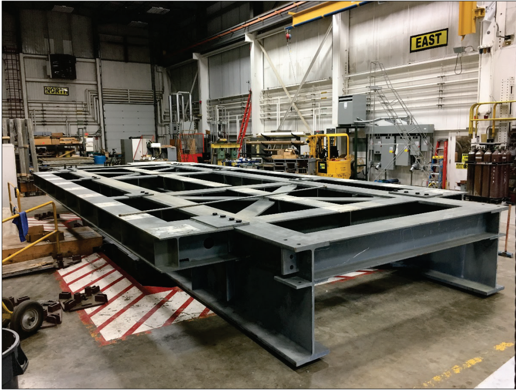
Figure 2. Test fixture bolted to the TESS shake table.
