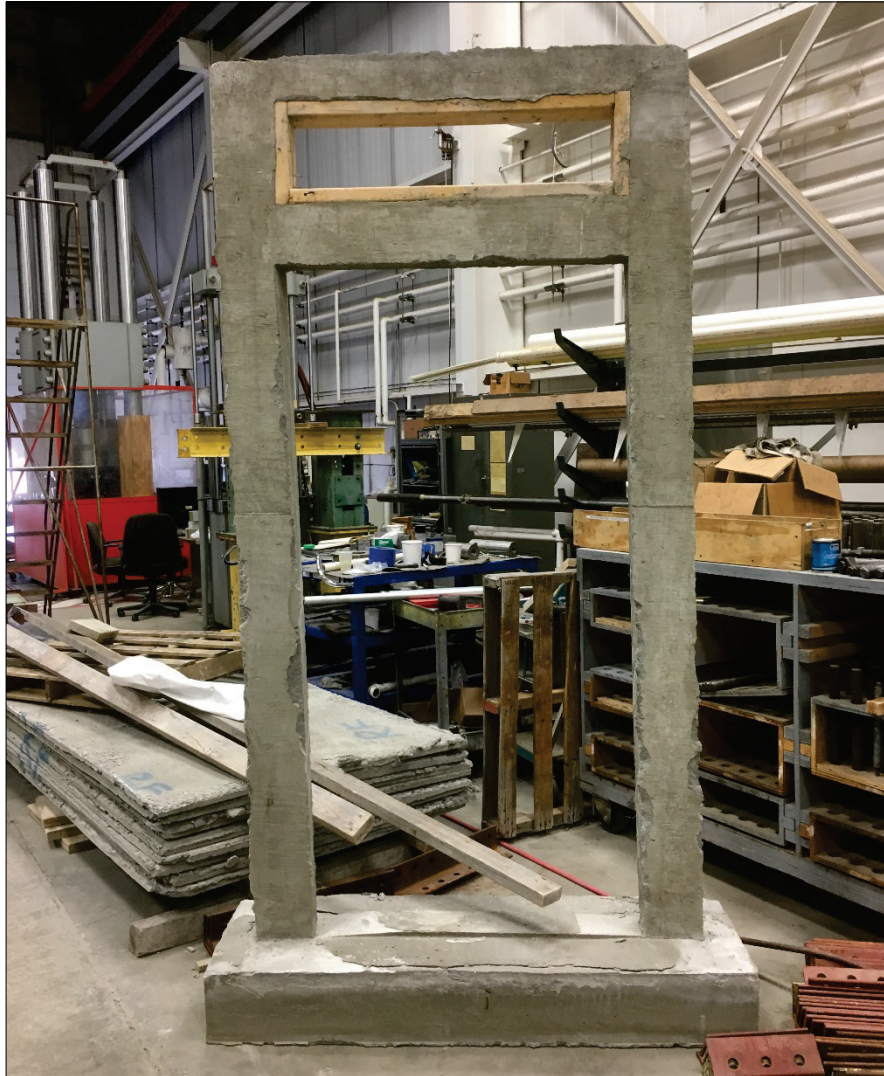
Figure 10. Door frame precast with a single footing.
