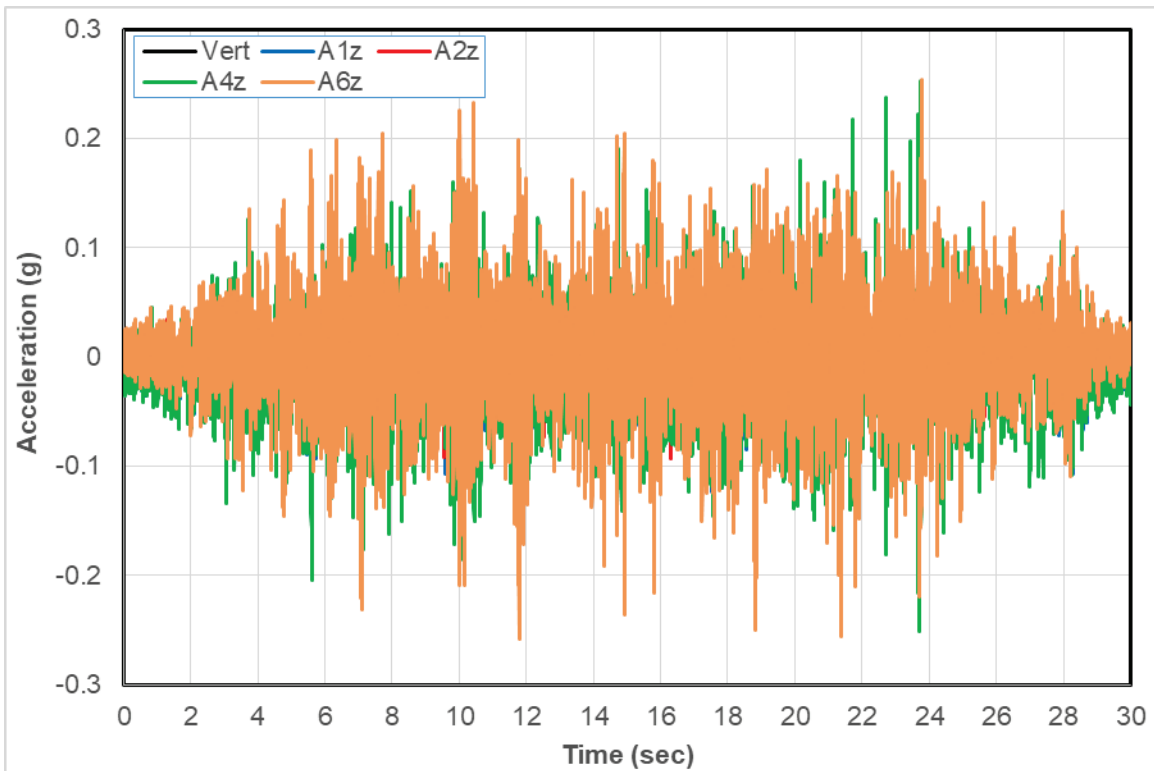
Figure C-3. Accelerations recorded in the Z-axis during the 10% seismic test.
