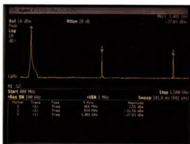
Figure 124. Spectral amplitudes at fundamental frequency (467 MHz), second harmonic frequency (934 MHz), and third harmonic frequency (1401 MHz).
