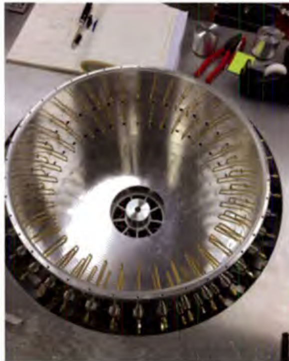
Figure 109. Cavity power combiner showing 80 loop antennas
