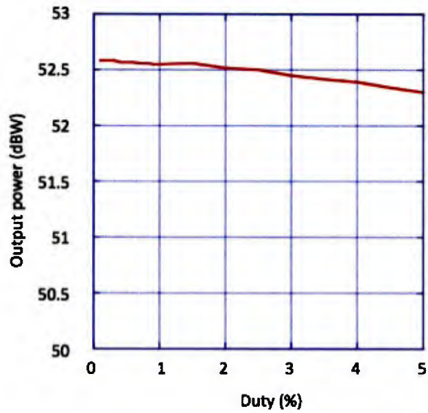
Figure 121. RF output power as functions of duty cycle varying from 0.1 % to 5 %
