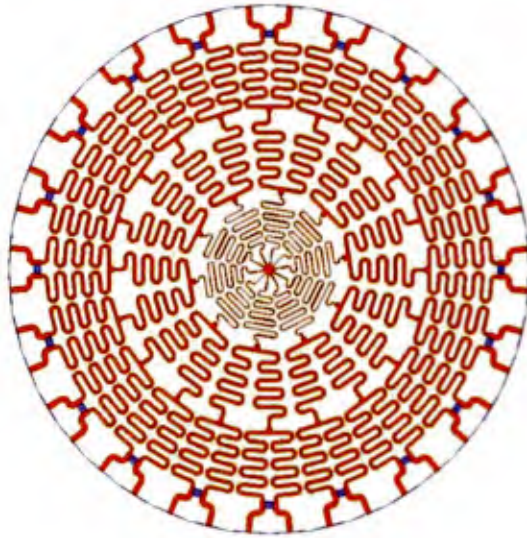
Figure 51. 40-way power divider consisting of a 10-way radial power divider and 2 stage 3-dB Wilkinson dividers.
