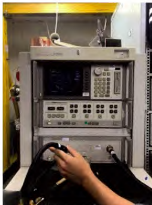
Figure 61. Photo showing a probe measurement technique using VNA
