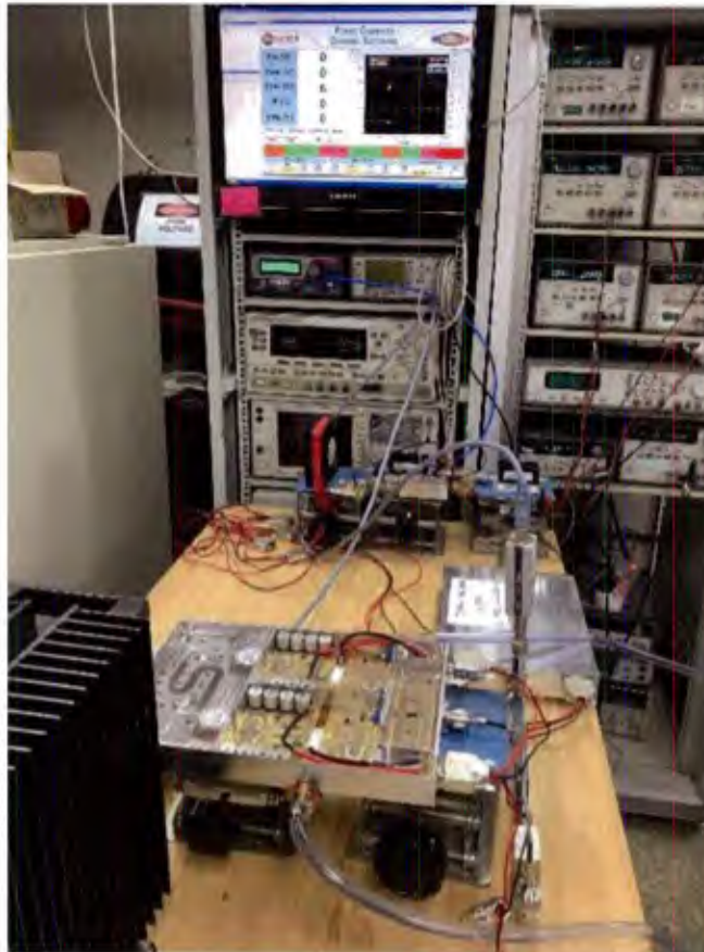
Figure 21. Experimental setup for testing 2 kW SSPA module
