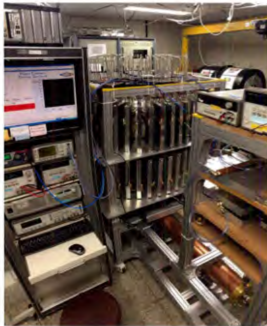
Figure 111. Photo of 80-way power combiner system, operating at low duty cycle (duty cycle = 0.1 %, PRF = 10 Hz, PW = 100 microseconds)
