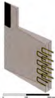
Figure 40. HFSS full model and symmetry model: (a) 80-way, (b) 120-way, and (c) 160-way power combiners
