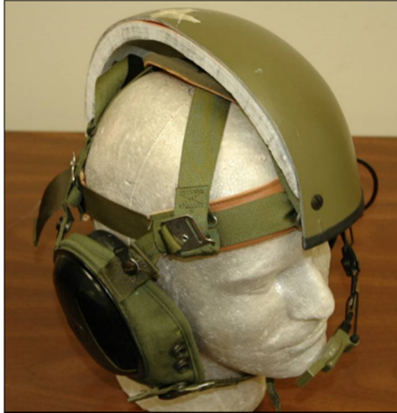
Figure 1. SPH-4 helmet cross section exposing the sling suspension fitting system.
