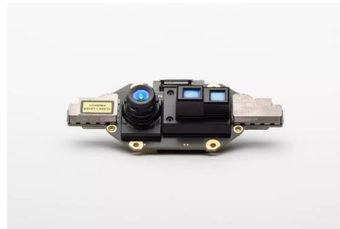
Figure 15: Depth Sensor common to HoloLens 2 and Kinect for Azure
