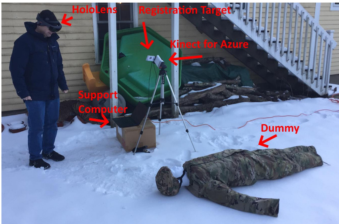
Figure 24: Outdoor testing with complete prototype system and dummy
