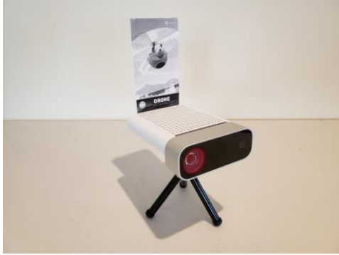
Figure 19: Azure Kinect with added Vuforia Registration Tag
