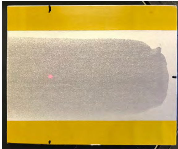
Figure 10. 75 \mu\text{m} layer of plain Al-Si-10Mg powder manually spread on Al-12Si substrate with a beveled steel blade.
