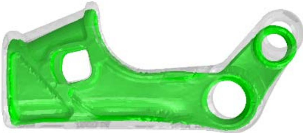
Figure 3.40 Deformed casting at room temperature.
