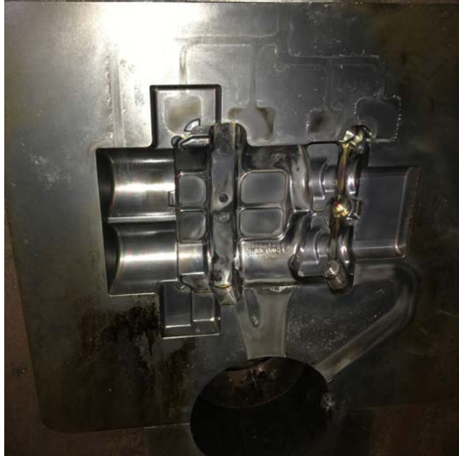
Figure 21 Photograph of the surface of the AlCrN coated die after the production of 11,652 shots
