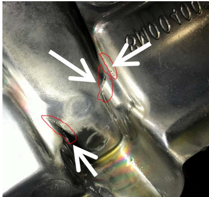
Figure 22: The highlighted locations in the die show the onset of minor heat checking
