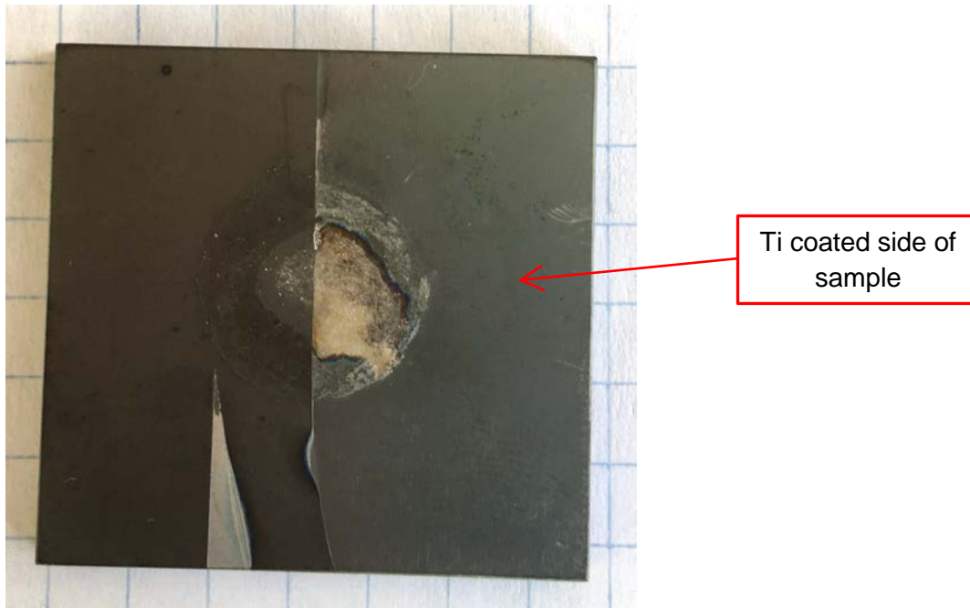
Figure 11a. Photograph of the AlCrN coated substrate, with a thin metallic layer of titanium on the right-hand side. The photograph shows the sample after the Aluminum Adhesion Test, indicating that the aluminum alloy stuck to the titanium-coated side of the sample, but not to the bare AlCrN coating
