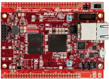
Figure 4-14. Integration concept for Draper electronics with photographs of MicroZed SOM and thermal control board.
