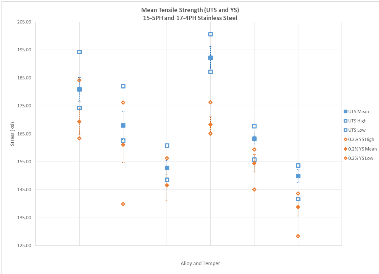
Figure 12. Tensile Properties of 15-5PH and 17-4PH Stainless Steel
