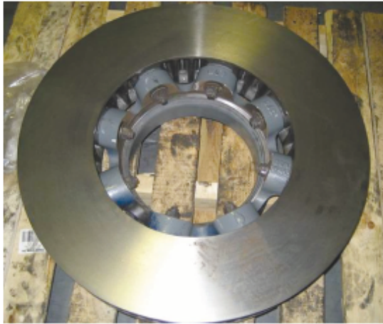
Figure 7. Hub mounted into cast iron brake disc rotor.
