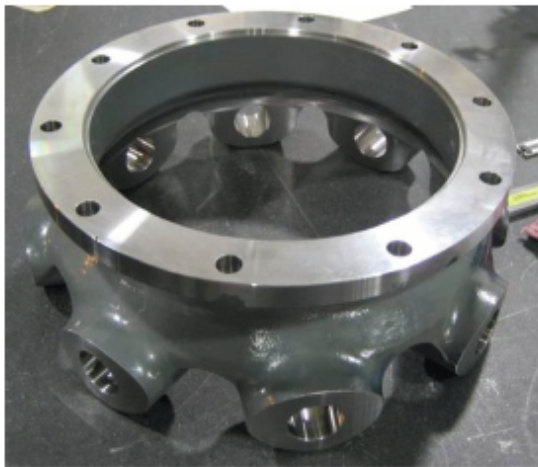
Figure 8. Cast steel hub after finish machining.
