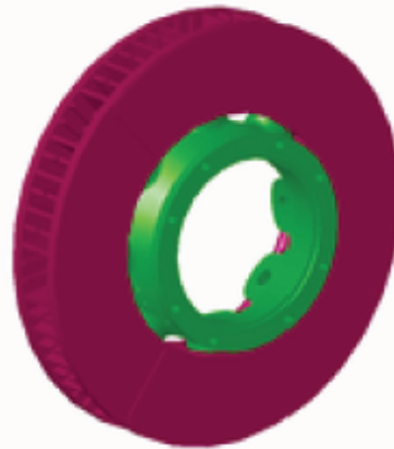
Figure 9. FEA model of the rotor disk with hub assembly.
