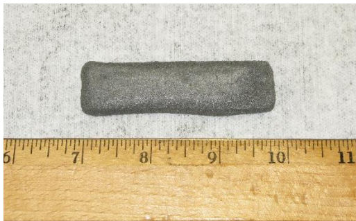
Fig. 6 Test bar produced using recycled 304 SS powder and Chihuahuan Desert sand (scale of ruler is inches)
