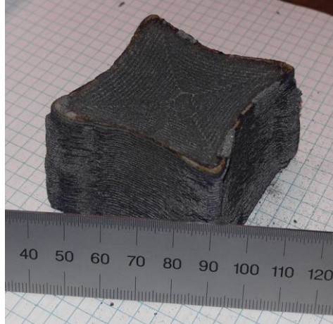
Fig. 3 First cube produced using hydrided Ti-6Al-4V powder in the OPL; visible is the surface layer that typically forms during sintering, while closer inspection reveals the layered structure generated in OPL (scale of ruler is in mm)
