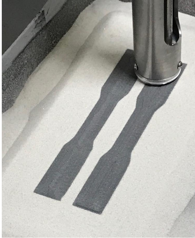
Fig. 7 Deposition of 15-cm-long dogbone tensile specimens using FeNiZr powder
