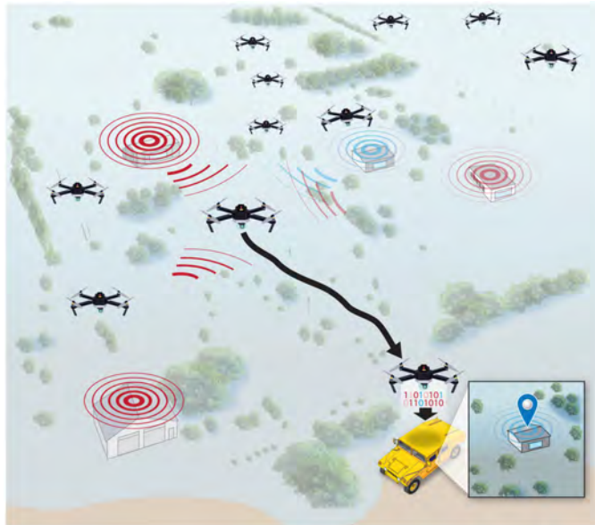
Figure 1. A rescue scenario where UAV sensors are trying to locate signals in the presence of interference. Each UAV in the distributed array collects and stores digital samples before returning to a hub where adaptive beamforming techniques are used to estimate the location of the signals.
