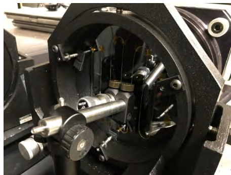
Figure 9. Close-up view of the back of the instrumented silicon wafer showing the micrometer fixture.
