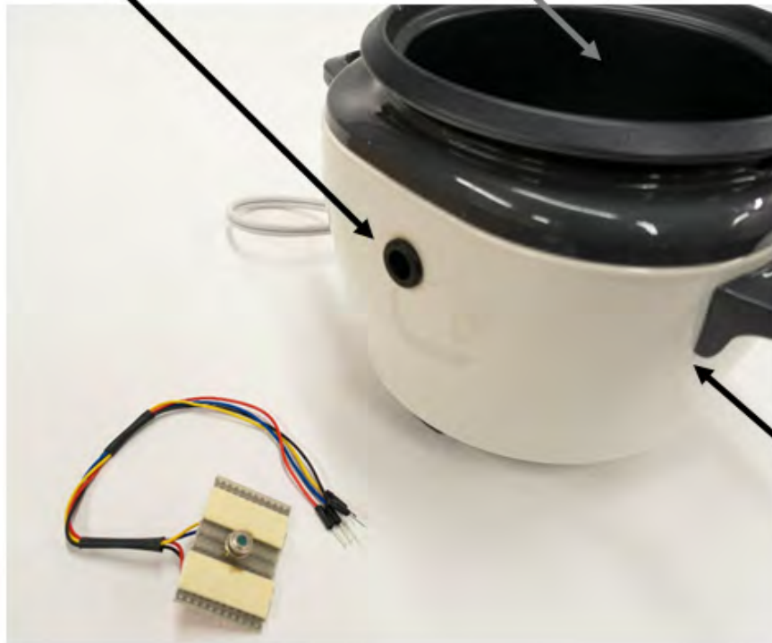
Figure 23. IR sensor and modified rice cooker.
