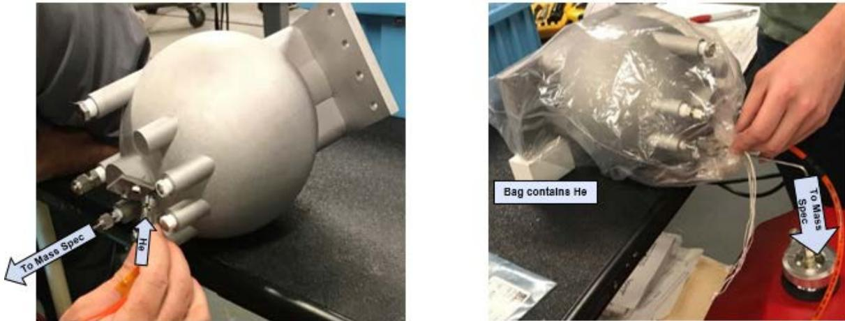
Figure 22: Leak check process.
