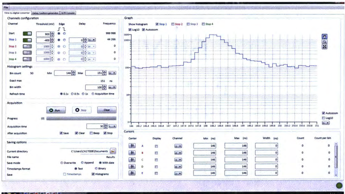
Figure 3: Histogram GUI example with TPSF from Human adipose tissue w/ 1cm perpendicular spacing w/105um fiber and Lumics laser diode using the setup from Figure 2
