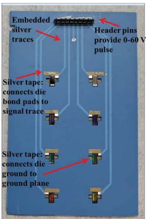
Figure 20. (Left) Photograph of the GFEA test structure for temporary electrical connections to the die for testing in vacuum and (right) photograph of the phosphor screen in the test chamber excited by a GFEA die.
