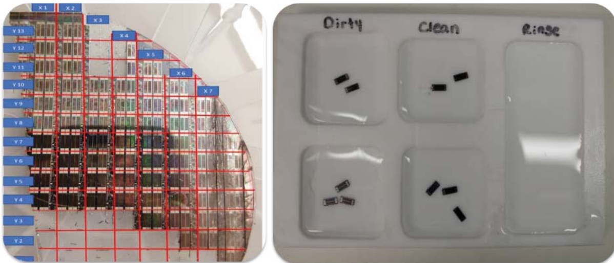
Figure 19. Photographs of (left) GFEA wafer section from MIT coated with resist and sawed into individual die and (right) photograph of the die strip containers where acetone is used in clean and dirty trays followed by a DI rinse.
